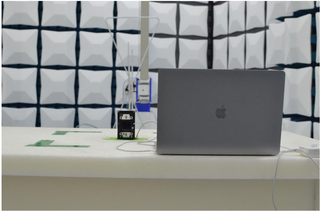
Figure 17: 30MHz-1GHz Test Setup (Rear View)
