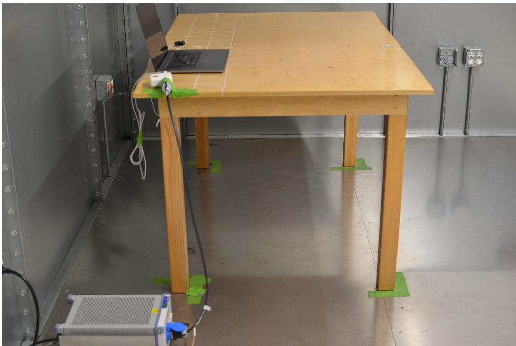
Figure 4: AC Line Conducted Emissions (Side View)
