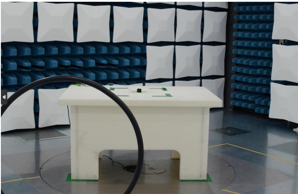
Figure 24: 9kHz-30MHz Test Setup (Front View)
