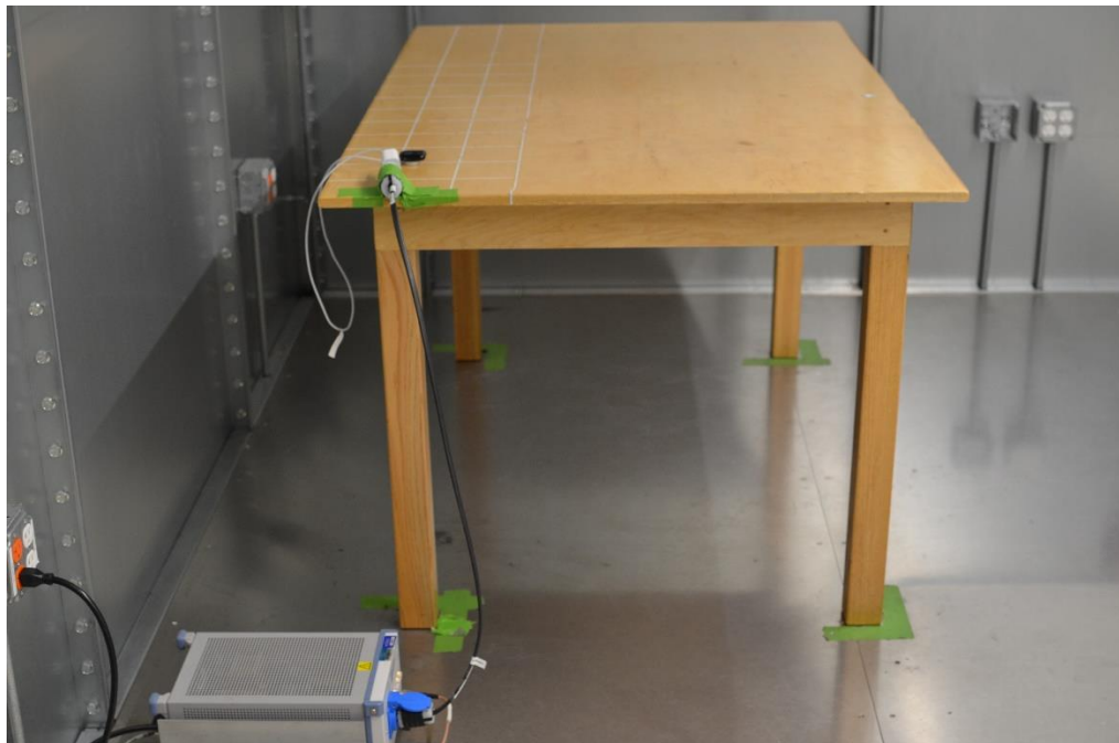
Figure 2: AC Line Conducted Emissions (Side View)
