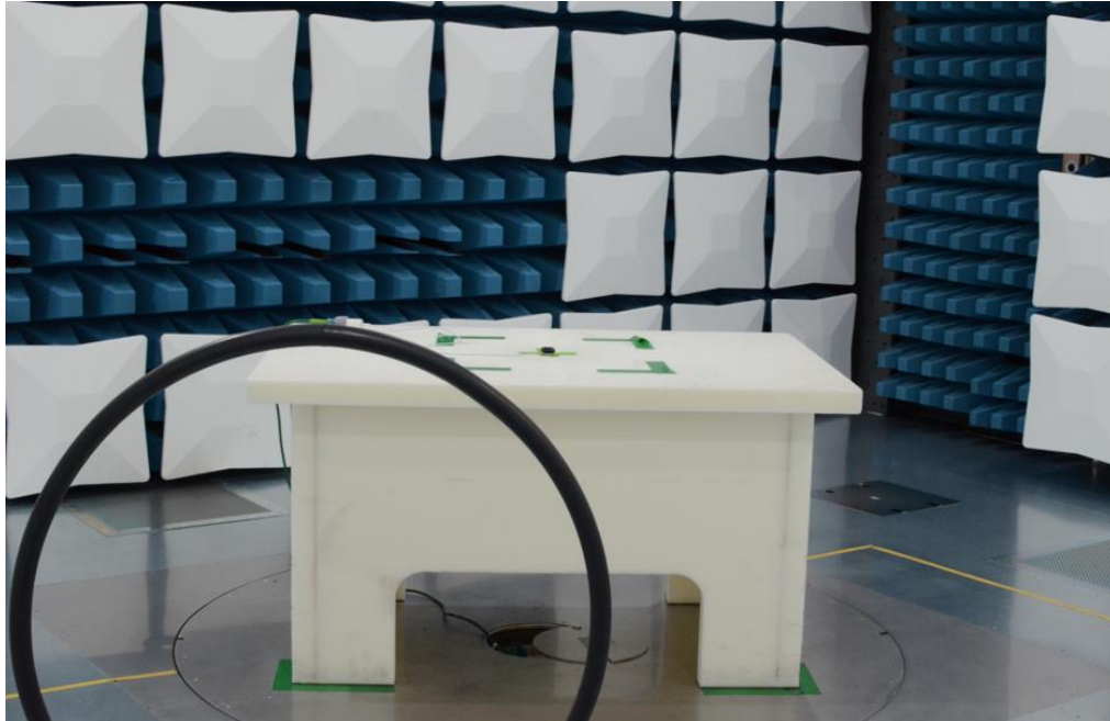
Figure 23: 9kHz-30MHz Test Setup (Front View)
