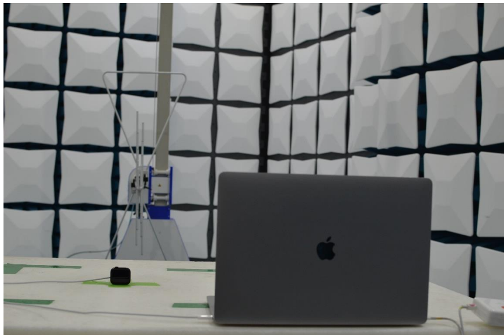
Figure 20: 30MHz-1GHz Test Setup (Rear View)
