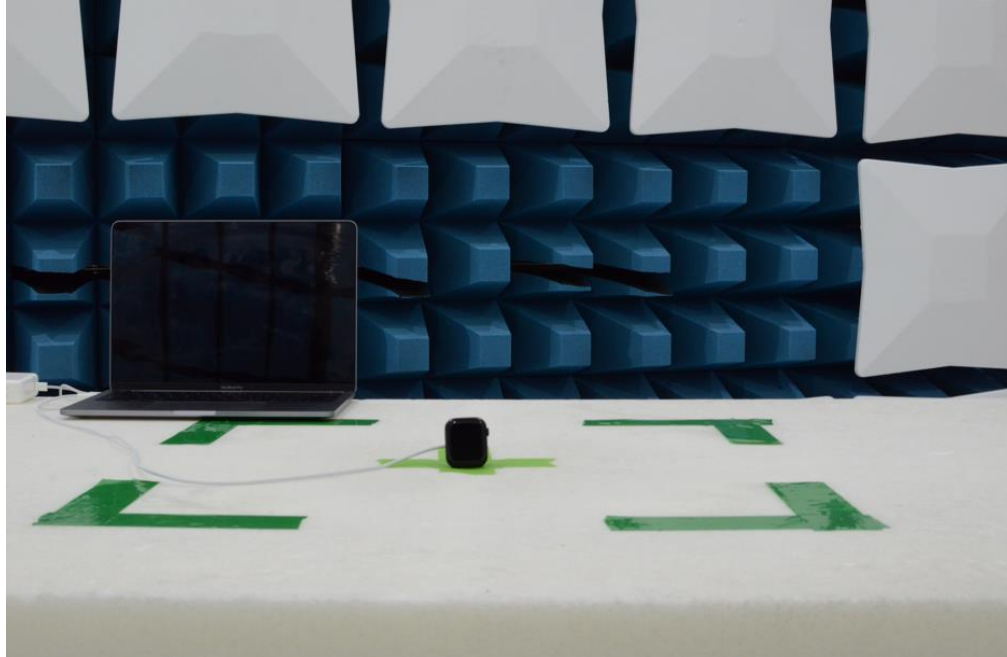
Figure 21: 30MHz-1GHz Test Setup (Front View)
