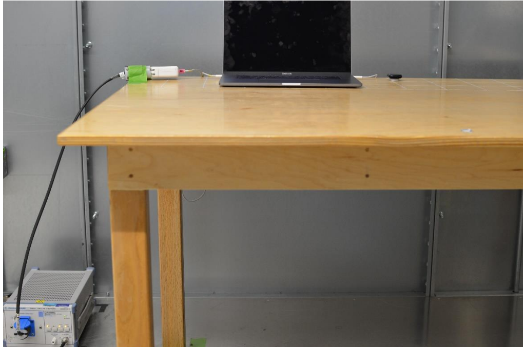
Figure 3: AC Line Conducted Emissions (Front View)
