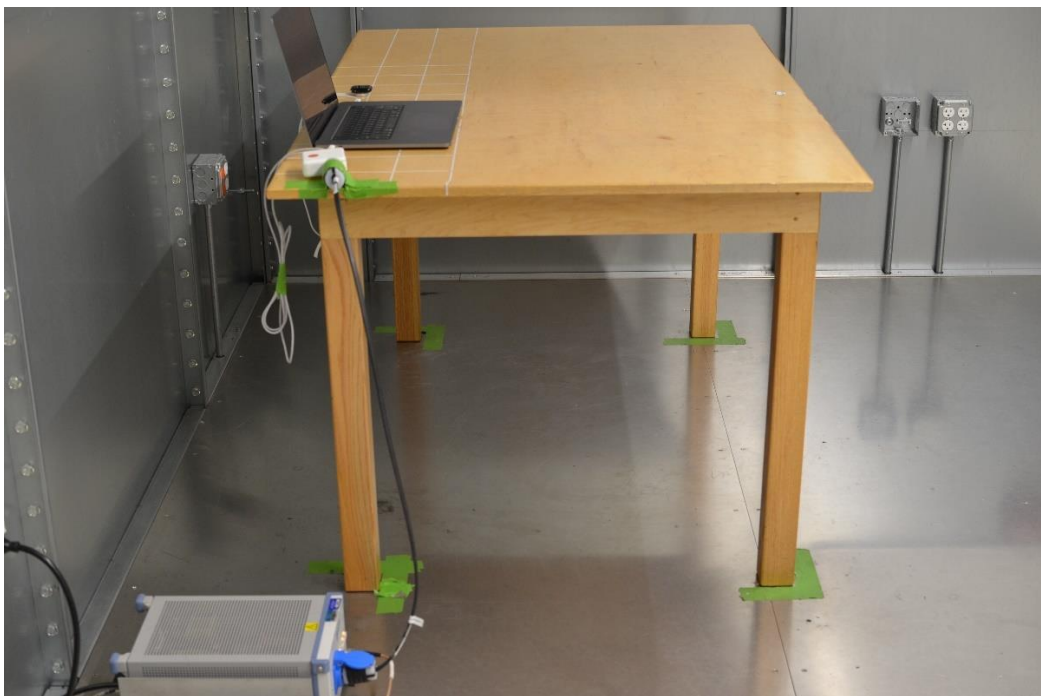
Figure 4: AC Line Conducted Emissions (Side View)
