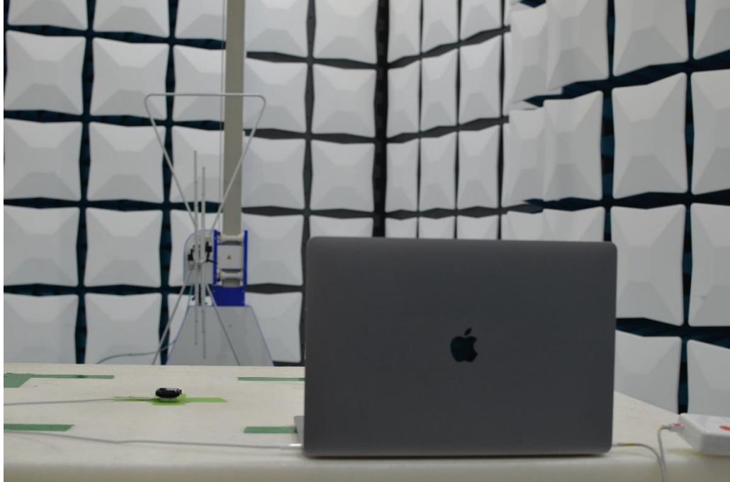
Figure 15: 30MHz-1GHz Test Setup (Rear View)
