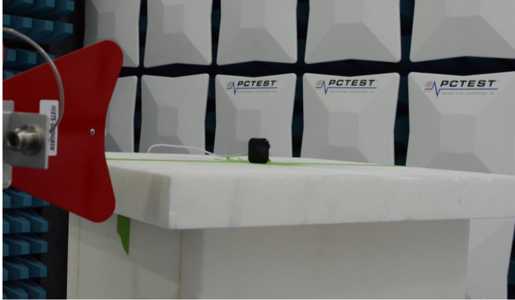
Figure7: Above 960MHz Test Setup
