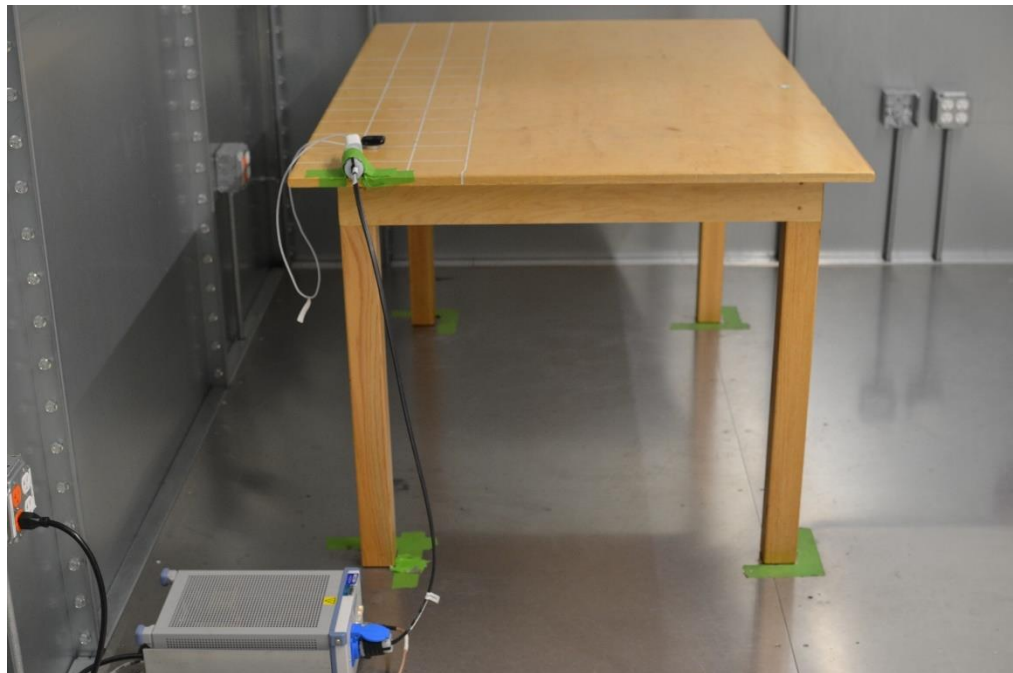
Figure 2: AC Line Conducted Emissions (Side View)
