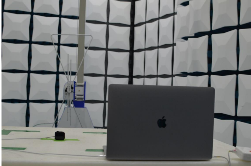
Figure 17: 30MHz-1GHz Test Setup (Rear View)
