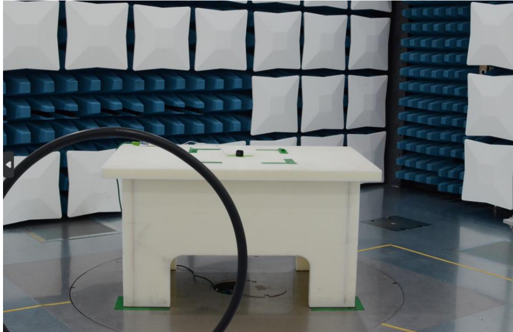
Figure 21: 9kHz-30MHz Test Setup (Front View)
