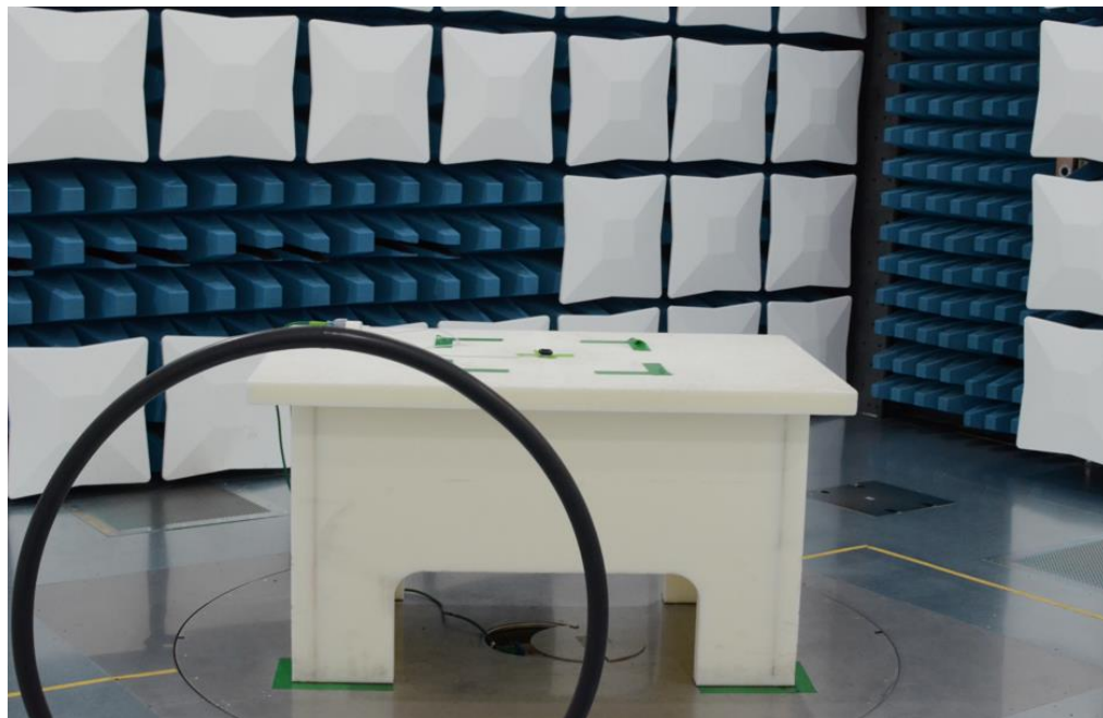
Figure 20: 9kHz-30MHz Test Setup (Front View)
