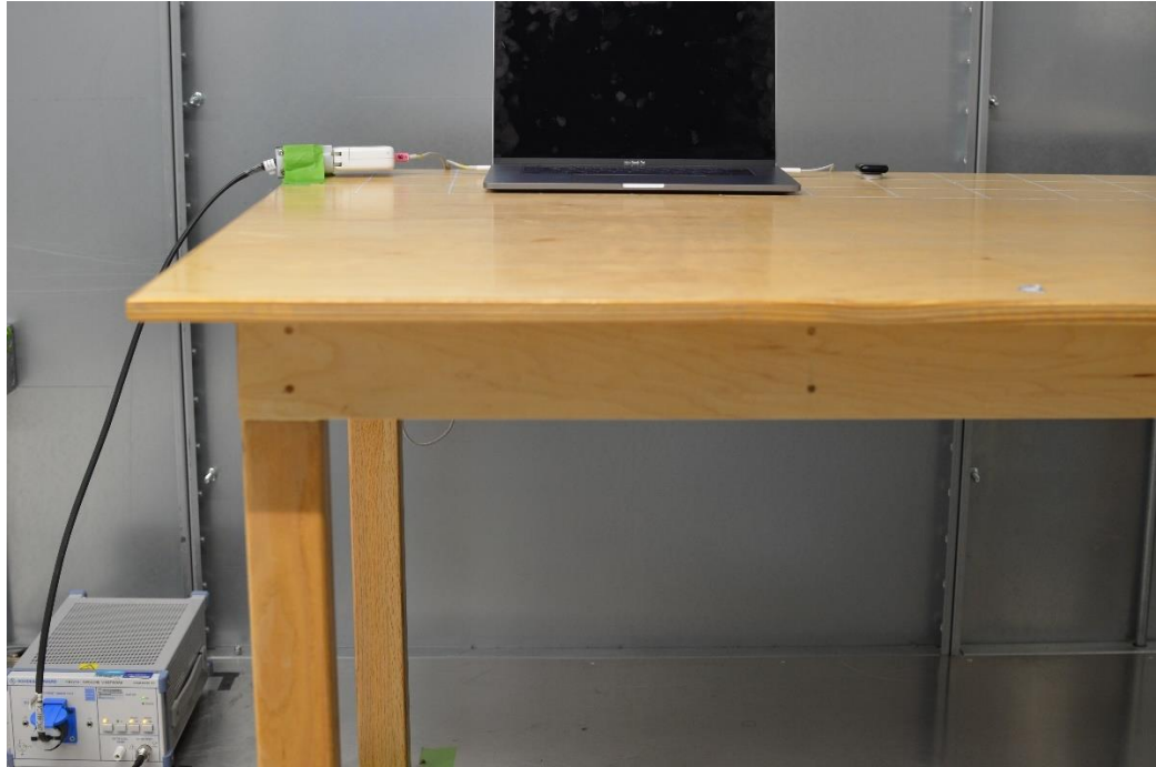
Figure 3: AC Line Conducted Emissions (Front View)
