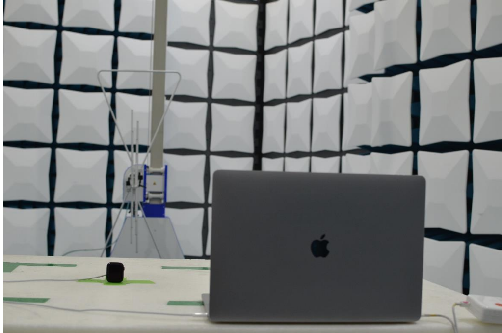
Figure 19: 30MHz-1GHz Test Setup (Rear View)
