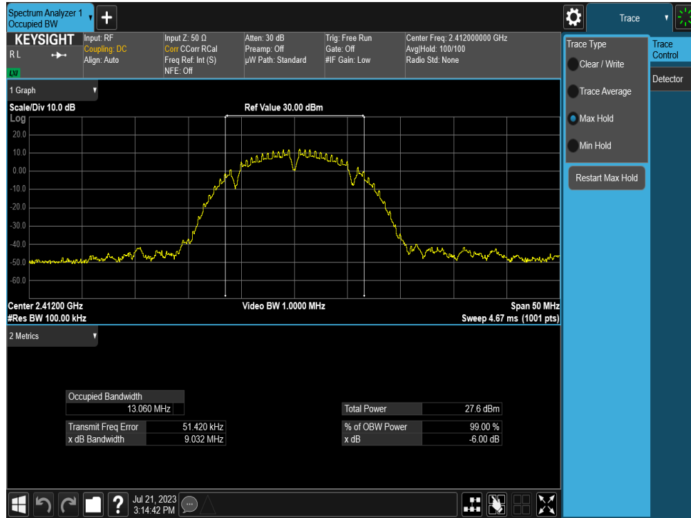
Plot 7-1. 6dB Bandwidth & 99% OBW Plot (802.11b – Ch. 1) – 1Mbps
