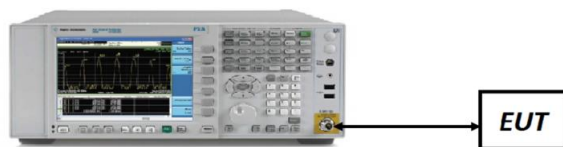
Figure 7-5. Test Instrument & Measurement Setup
