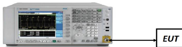
Figure 7-1. Test Instrument & Measurement Setup
