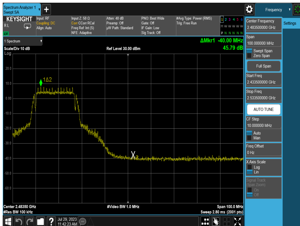
Plot 7-33. Band Edge Plot (802.11g – Ch. 9) – 6Mbps
