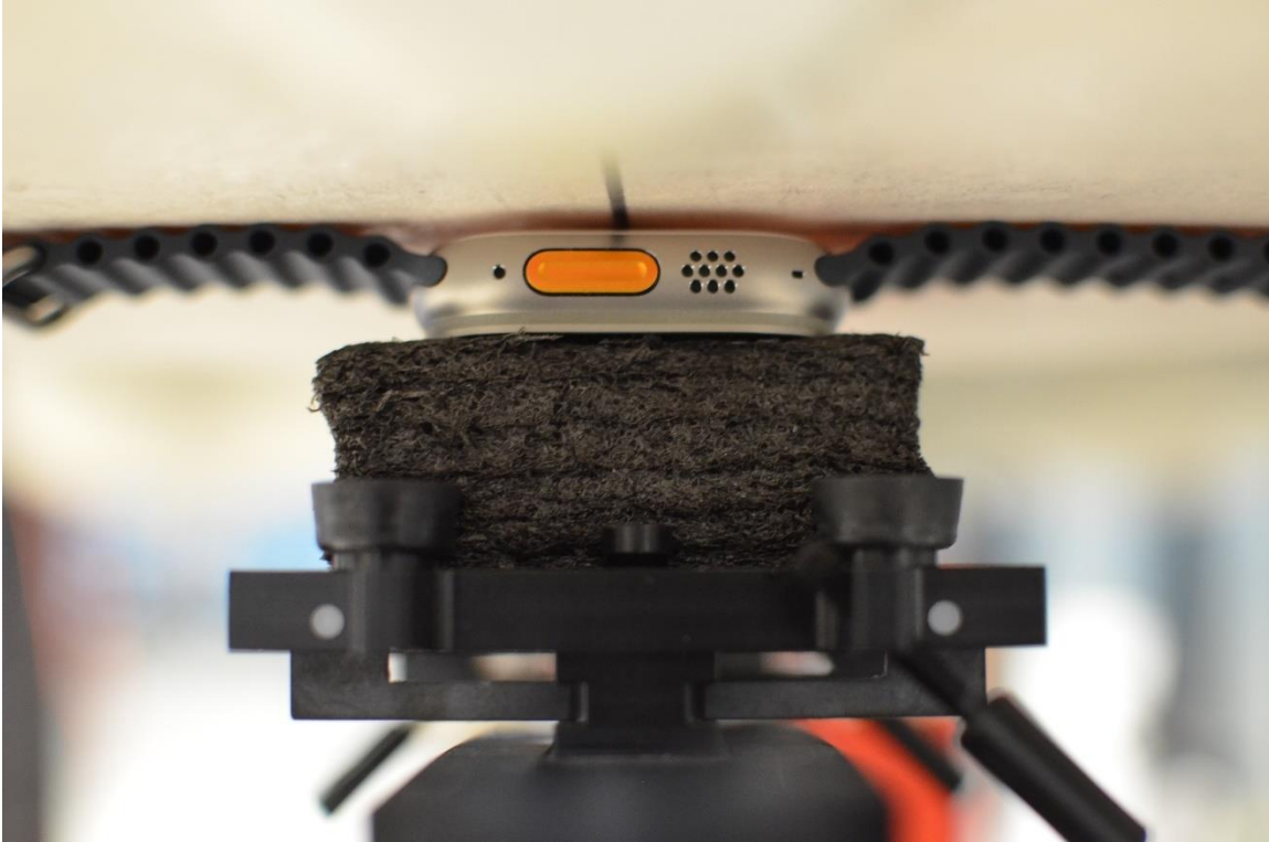
SAR Test Setup Photo 4: Titanium with Sport Wristband, Extremity, Back Side at 0.0 cm
