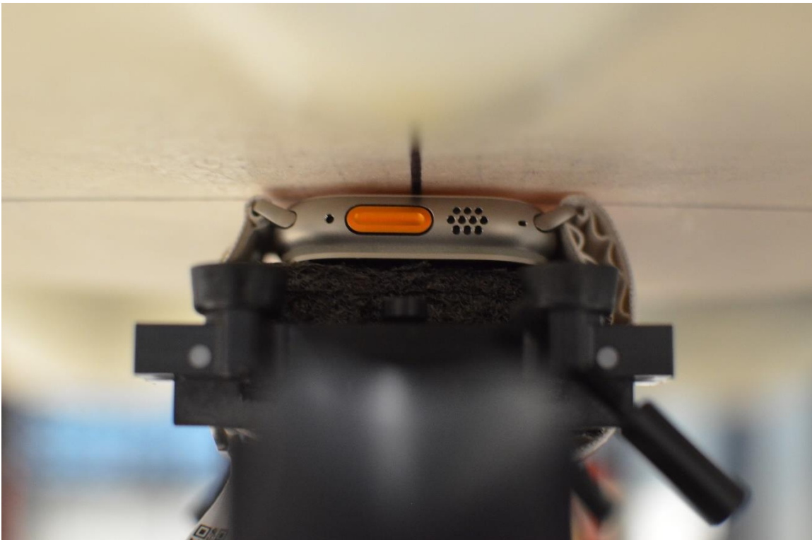
SAR Test Setup Photo 5: Titanium with Fabric Wristband, Extremity, Back Side at 0.0 cm
