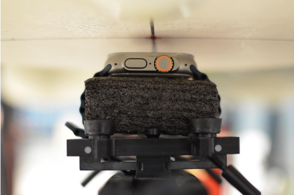
SAR Test Setup Photo 1: Titanium with Sport Wristband, Head, Front Side at 1.0 cm
