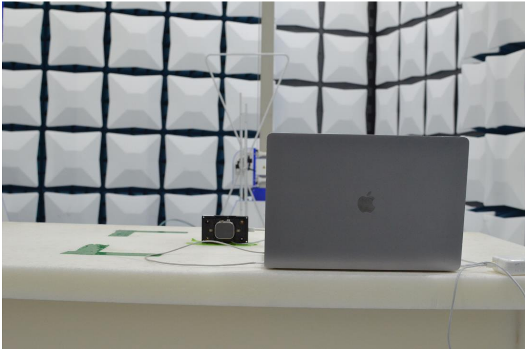
Figure 15: 30MHz-1GHz Test Setup (Rear View)
