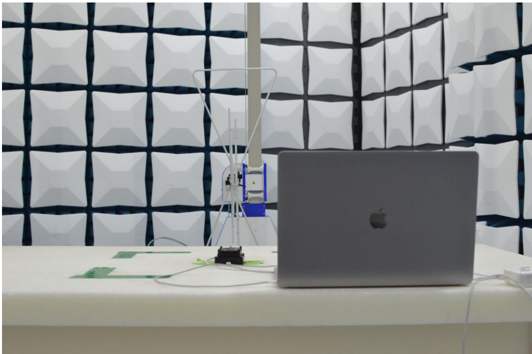
Figure 13: 30MHz-1GHz Test Setup (Rear View)
