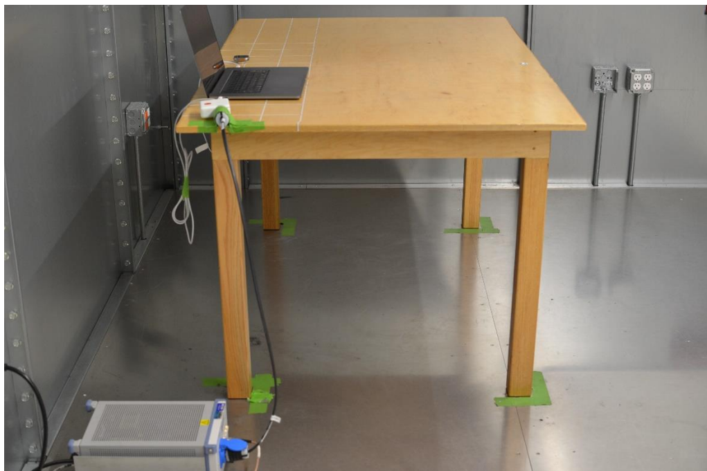
Figure 4: AC Line Conducted Emissions (Side View)
