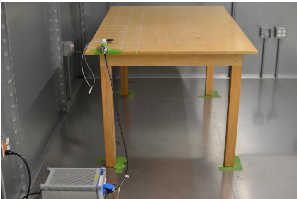
Figure 2: AC Line Conducted Emissions (Side View)
