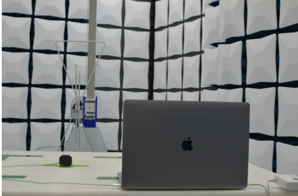
Figure 17: 30MHz-1GHz Test Setup (Rear View)
