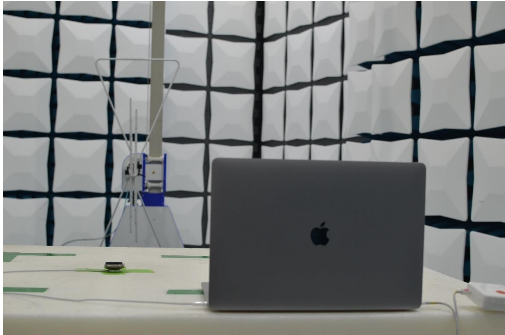
Figure 15: 30MHz-1GHz Test Setup (Rear View)
