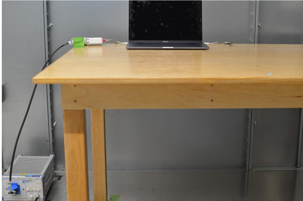
Figure 3: AC Line Conducted Emissions (Front View)
