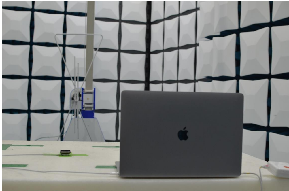
Figure 18: 30MHz-1GHz Test Setup (Rear View)
