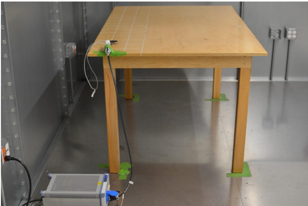
Figure 2: AC Line Conducted Emissions (Side View)
