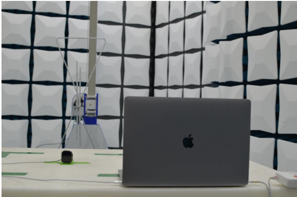
Figure 22: 30MHz-1GHz Test Setup (Rear View)
