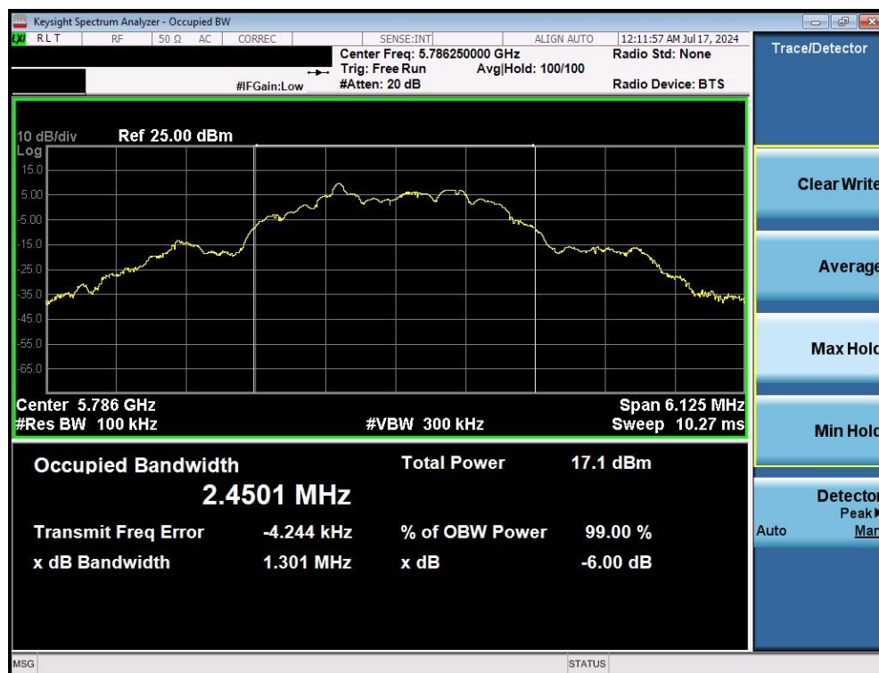
Plot 7-5. 6dB BW & 99% OBW (O-QPSK, 5786.25MHz, 500kpbs)
