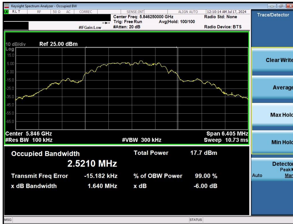
Plot 7-3. 6dB BW & 99% OBW (O-QPSK, 5846.25MHz, 250kbps)
