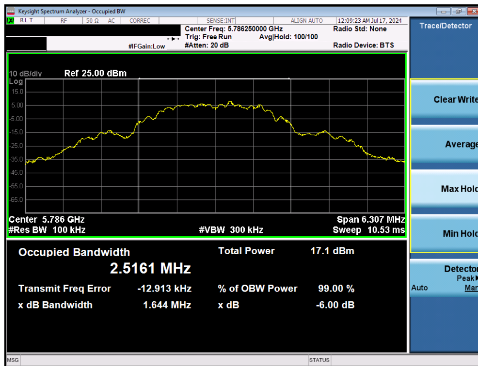
Plot 7-2. 6dB BW & 99% OBW (O-QPSK, 5786.25MHz, 250kpbs)
