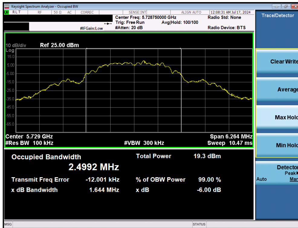
Plot 7-1. 6dB BW & 99% OBW (O-QPSK, 5728.75MHz, 250kpbs)
