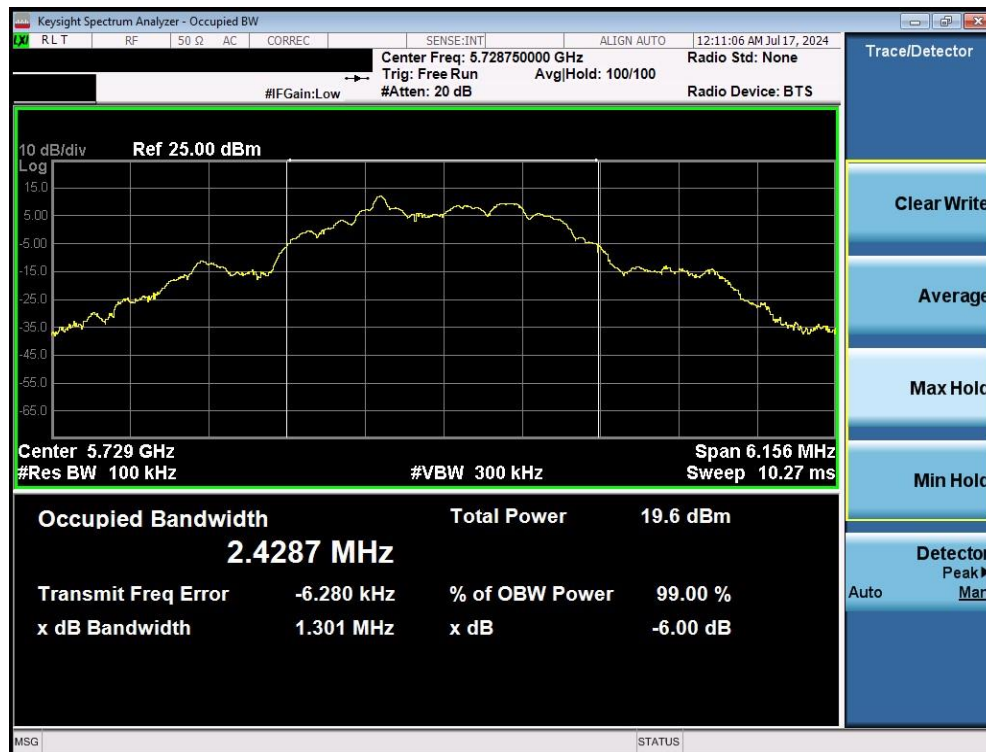
Plot 7-4. 6dB BW & 99% OBW (O-QPSK, 5728.75MHz, 500kbps)
