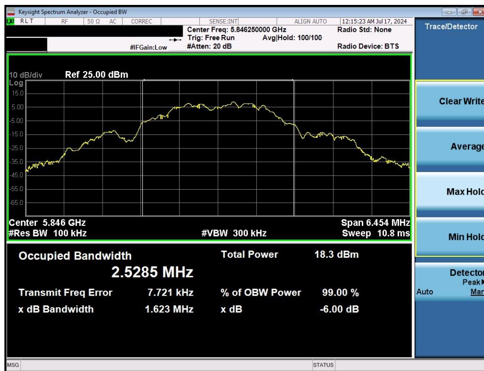
Plot 7-9. 6dB BW & 99% OBW (O-QPSK, 5846.25MHz, 1000kbps)
