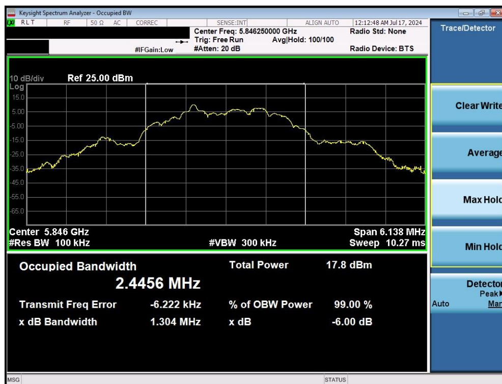
Plot 7-6. 6dB BW & 99% OBW (O-QPSK, 5846.25MHz, 500kpbs)
