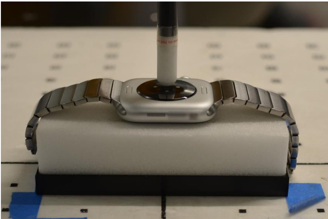
Near Field Power Density Test Setup Photo 12: Aluminum with Metal Links Wristband, Extremity, Back Side at 0.2 cm
