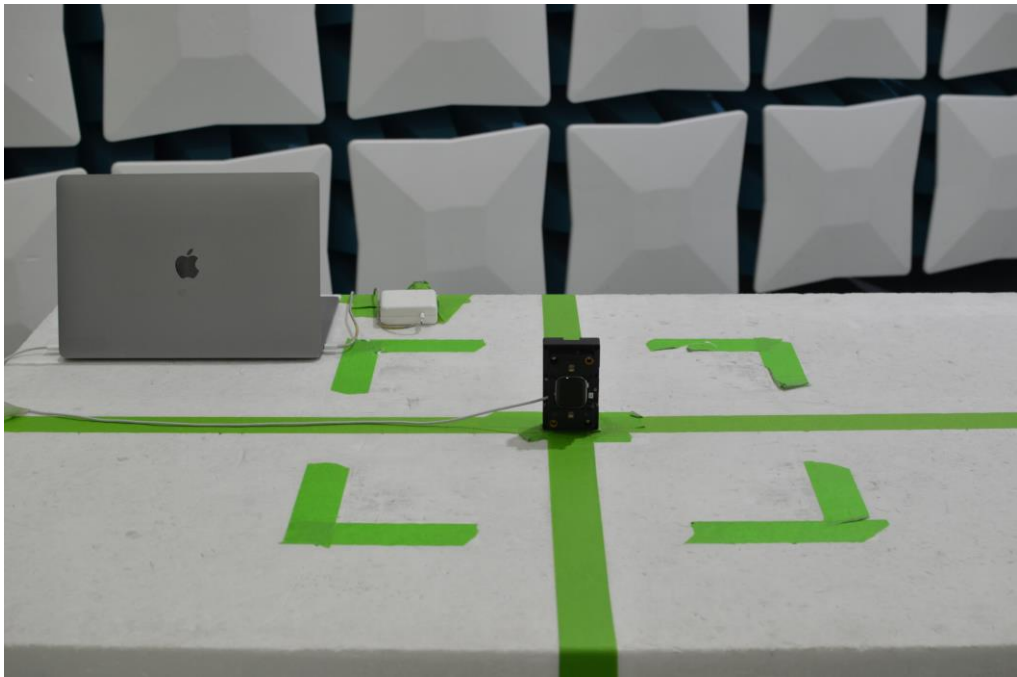
Figure 16: 30MHz-1GHz Test Setup (Front View)
