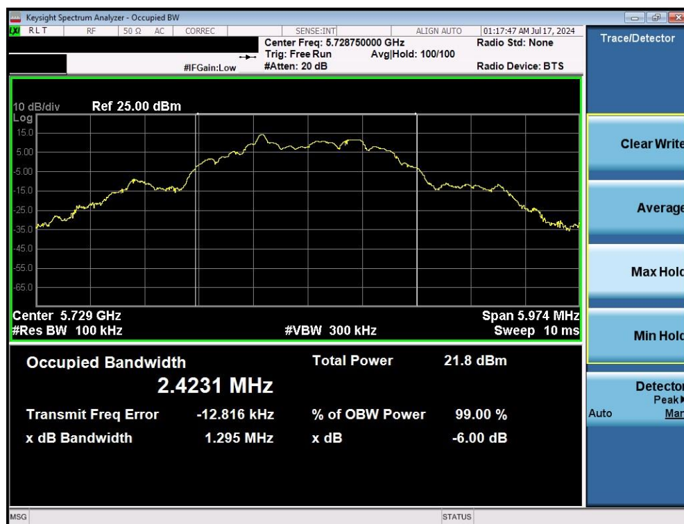
Plot 7-4. 6dB BW & 99% OBW (O-QPSK, 5728.75MHz, 500kbps)
