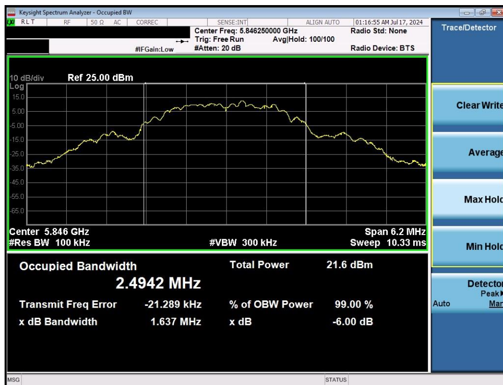
Plot 7-3. 6dB BW & 99% OBW (O-QPSK, 5846.25MHz, 250kbps)
