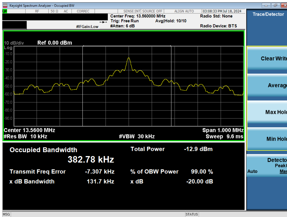
Plot 7-4. 20dB and 99% Bandwidth Plot (Reader 10% ASK 1 out of 4)
