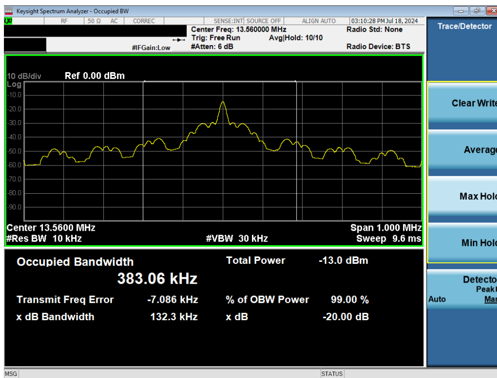
Plot 7-5. 20dB and 99% Bandwidth Plot (Reader 10% ASK 1 out of 125)
