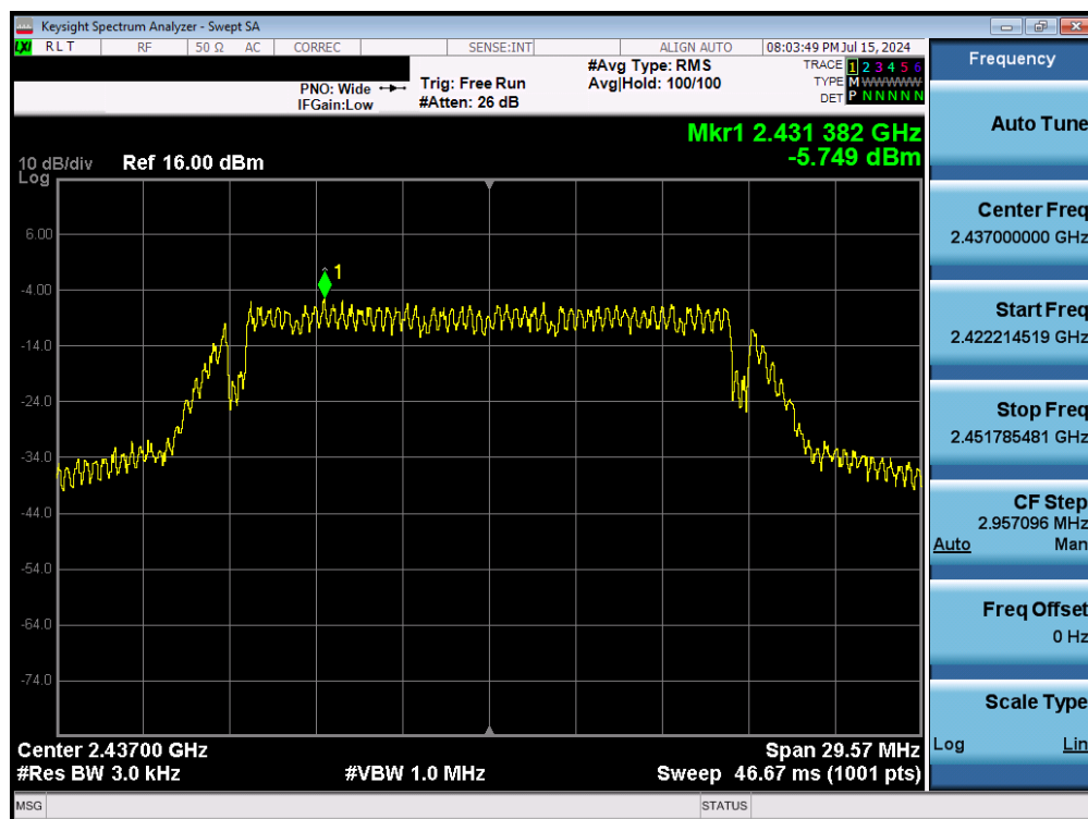
Plot 7-17. Power Spectral Density Plot (802.11g – Ch. 6) – 6Mbps
