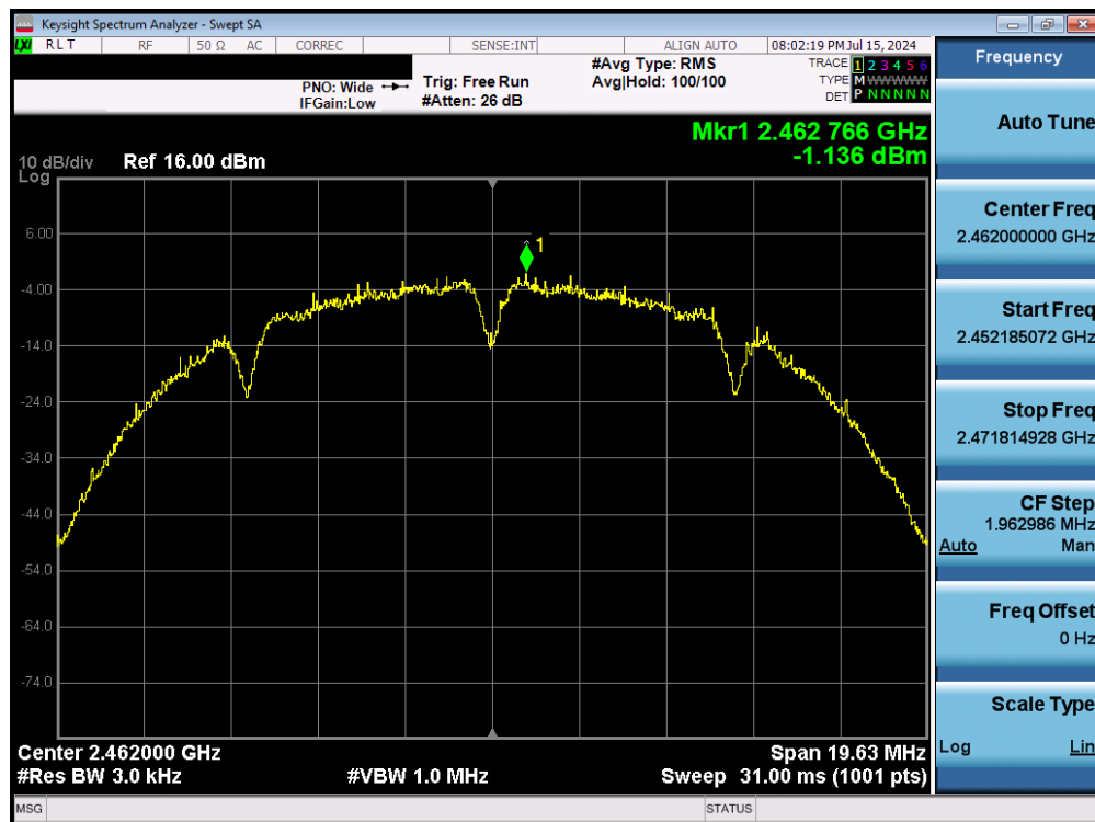
Plot 7-15. Power Spectral Density Plot (802.11b – Ch. 11) – 1Mbps
