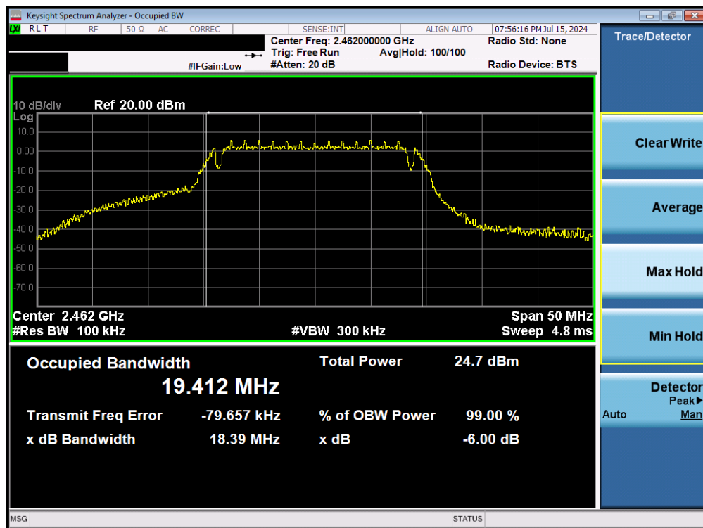
Plot 7-6. 6 dB BW and 99% OBW Plot (802.11g – Ch. 11) – 6Mbps
