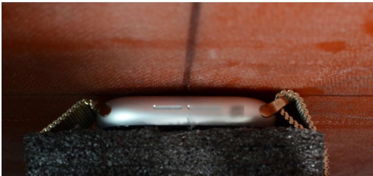
NFC Test Setup Photo 9: Aluminum with Metal Loops Wristband, Extremity, Back Side at 0.0 cm
