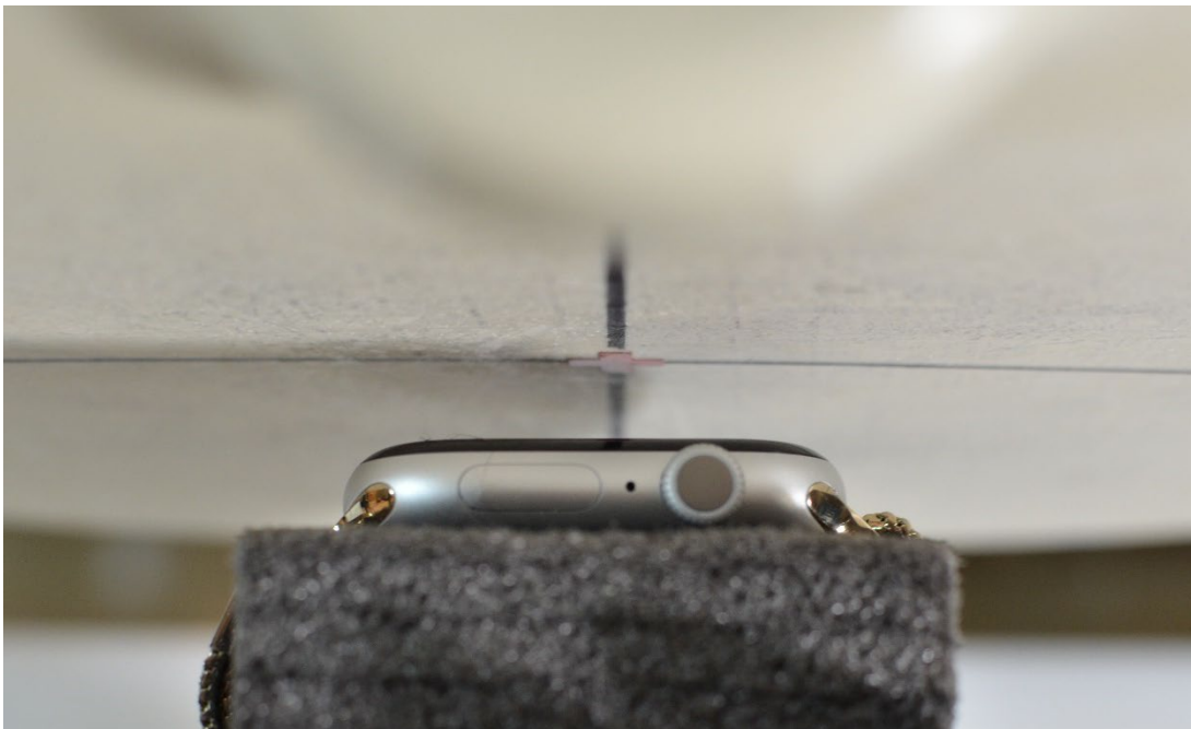
SAR Test Setup Photo 3: Aluminum with Metal Loops Wristband, Head, Front Side at 1.0 cm
