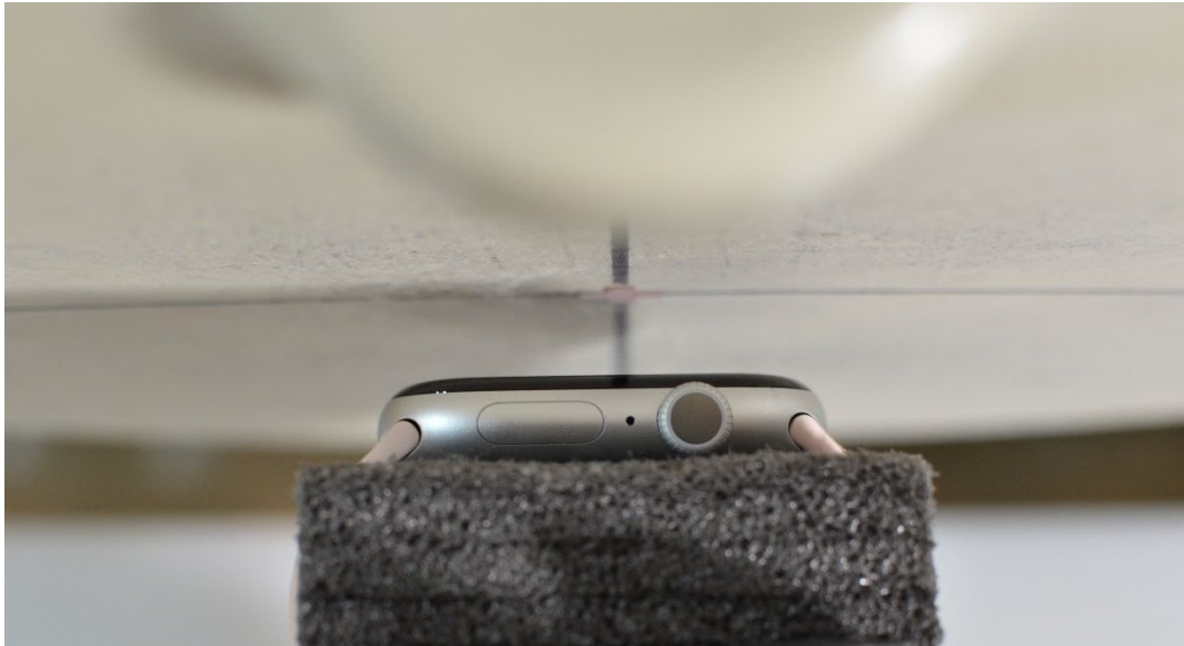
SAR Test Setup Photo 1: Aluminum with Sport Wristband, Head, Front Side at 1.0 cm
