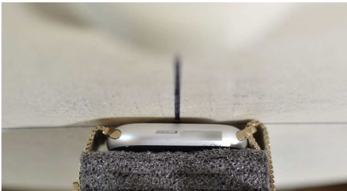
SAR Test Setup Photo 6: Aluminum with Metal Loops Wristband, Extremity, Back Side at 0.0 cm
