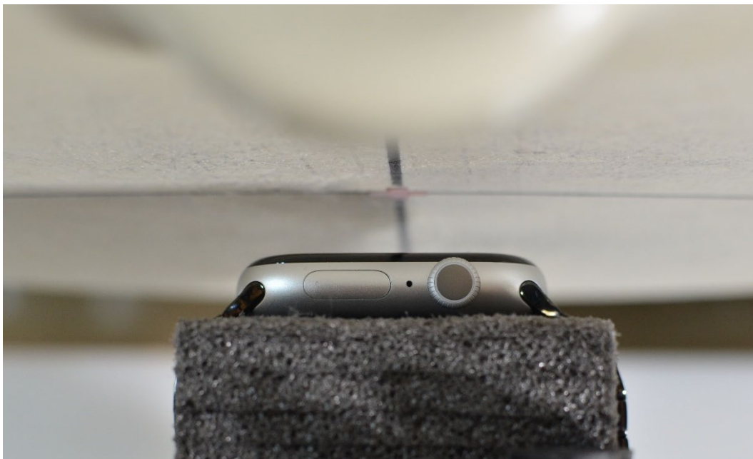
SAR Test Setup Photo 2: Aluminum with Metal Links Wristband, Head, Front Side at 1.0 cm
