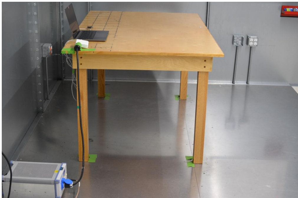
Figure 4: AC Line Conducted Emissions (Side View)
