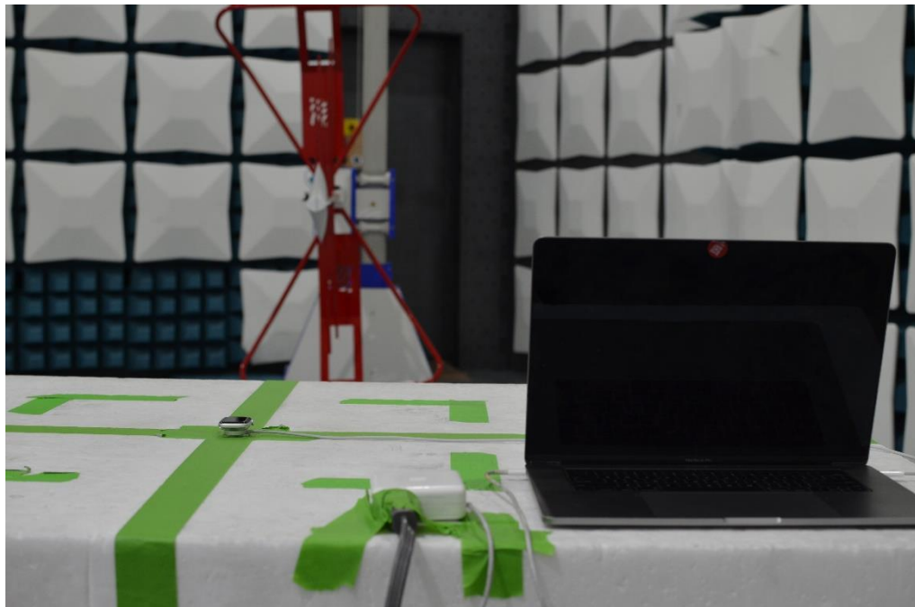
Figure 14: 30MHz-1GHz Test Setup (Rear View)
