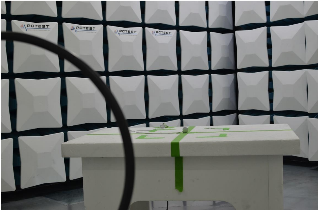
Figure 21: 9kHz-30MHz Test Setup (Front View)
