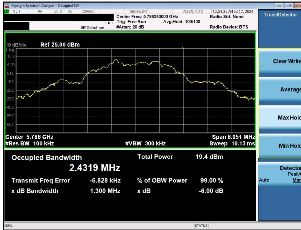
Plot 7-5. 6dB BW & 99% OBW (O-QPSK, 5786.25MHz, 500kpbs)
