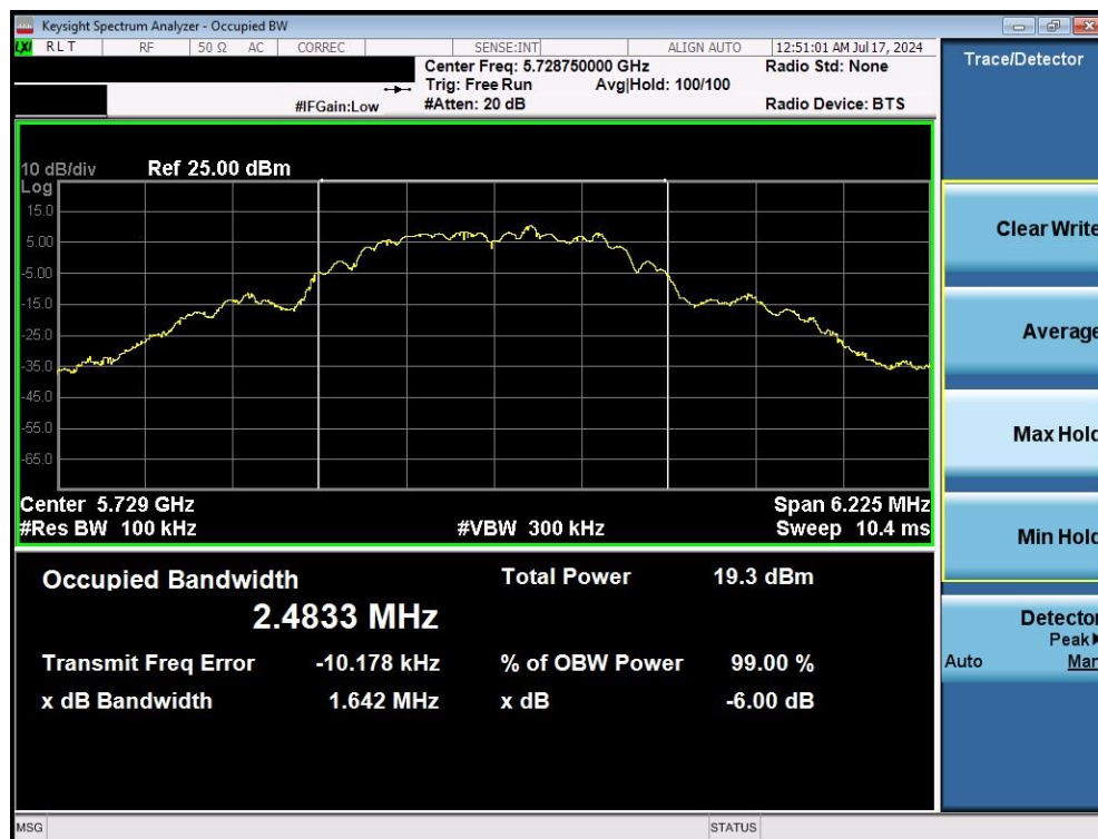
Plot 7-1. 6dB BW & 99% OBW (O-QPSK, 5728.75MHz, 250kpbs)
