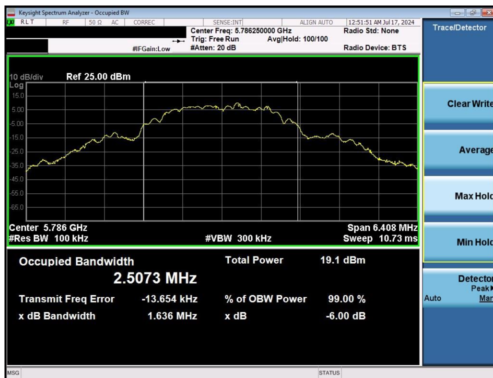
Plot 7-2. 6dB BW & 99% OBW (O-QPSK, 5786.25MHz, 250kpbs)
