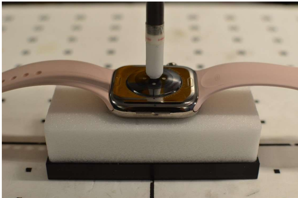
Near Field Power Density Test Setup Photo 23 – Titanium with Sports Wristband, Extremity, Back side at 2mm
