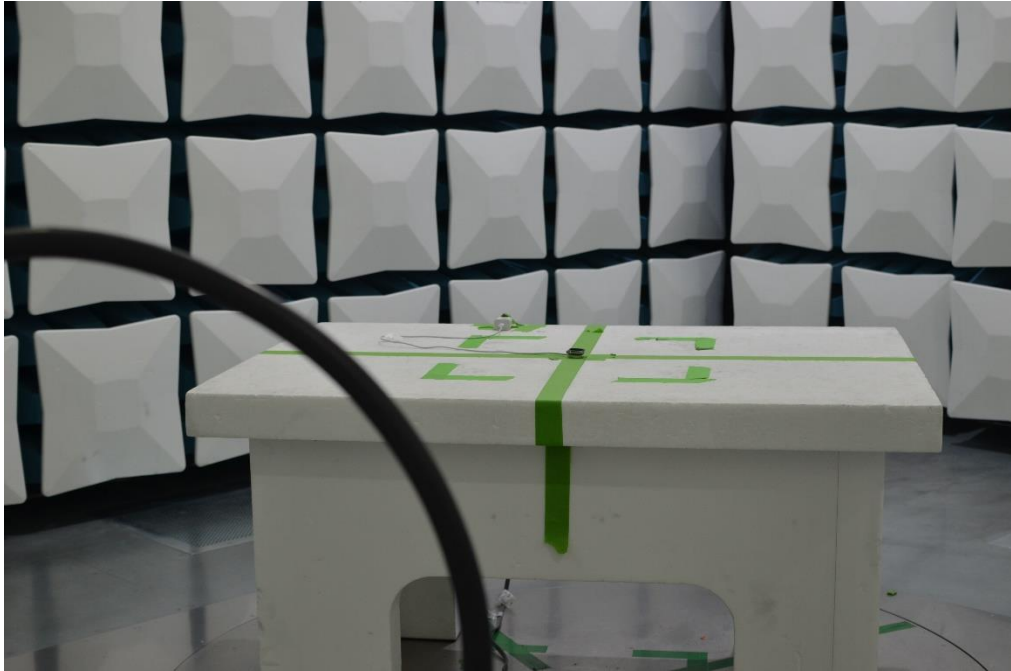
Figure 23: 9kHz-30MHz Test Setup (Front View)
