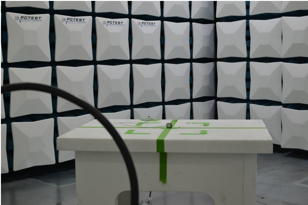
Figure 24: 9kHz-30MHz Test Setup (Front View)
