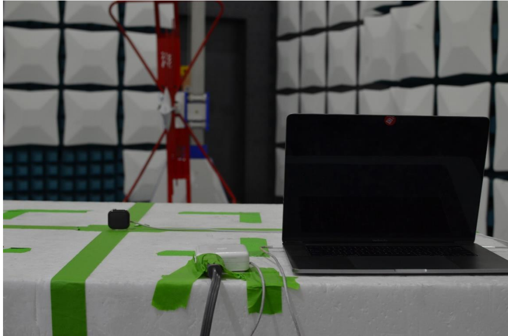
Figure 17: 30MHz-1GHz Test Setup (Rear View)
