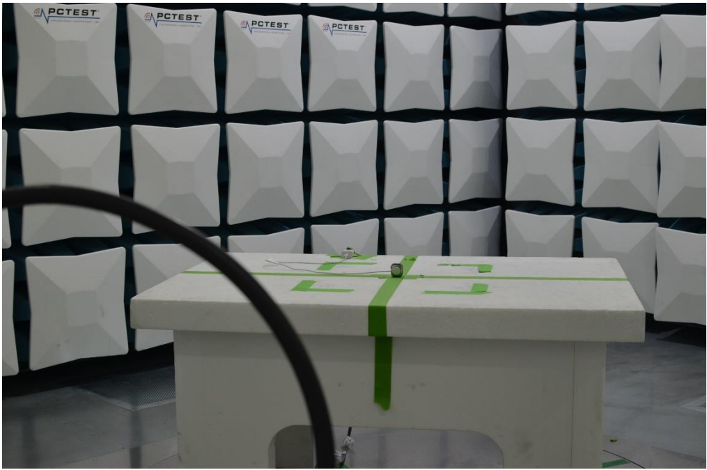
Figure 22: 9kHz-30MHz Test Setup (Front View)
