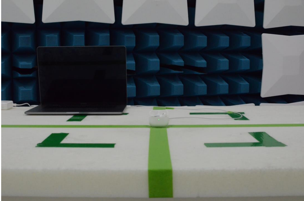
Figure 19: 30MHz-1GHz Test Setup (Front View)
