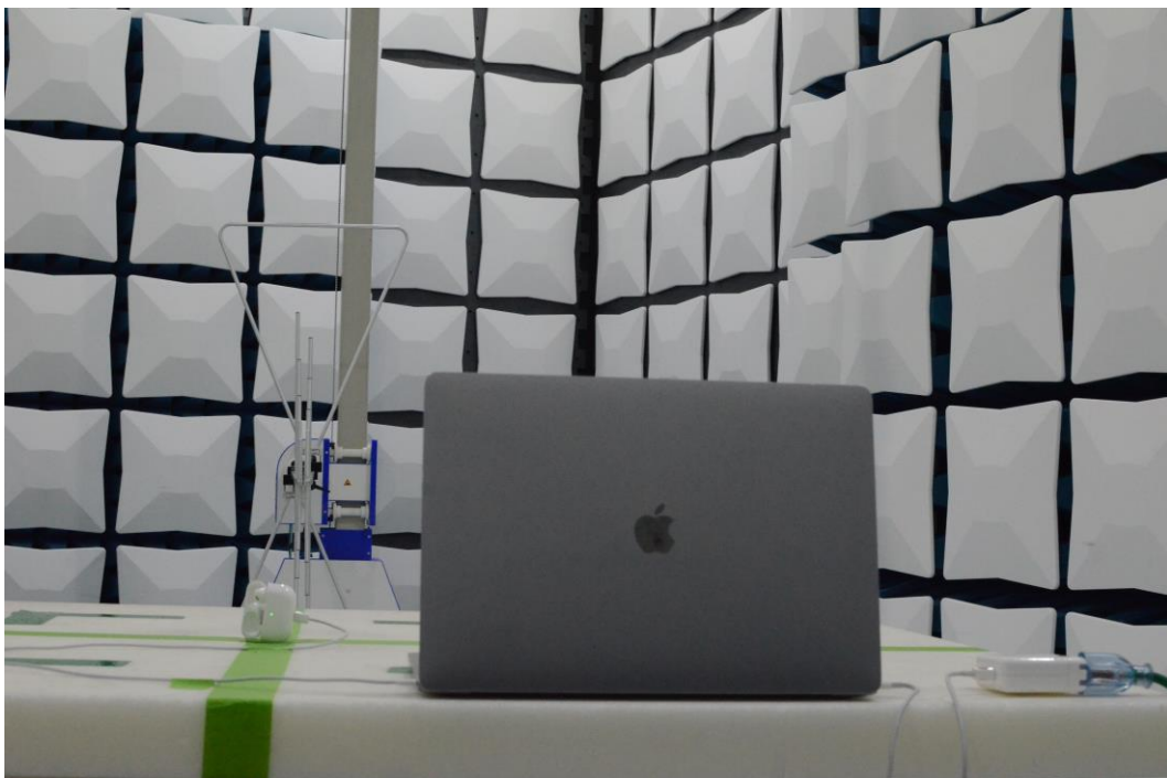
Figure 22: 30MHz-1GHz Test Setup (Rear View)
