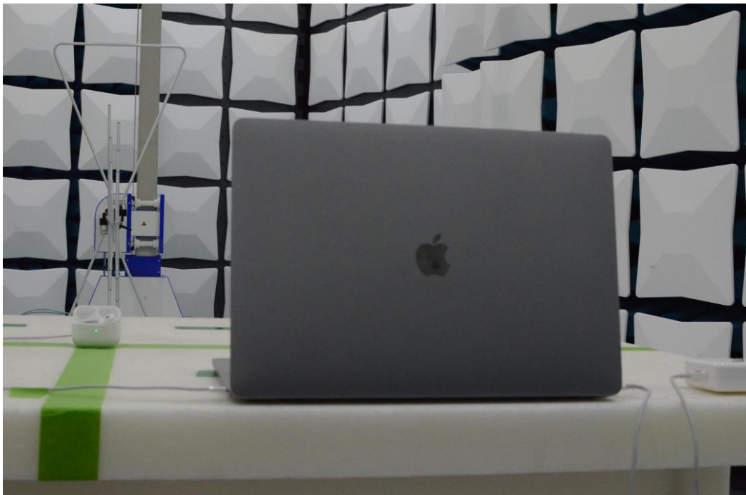
Figure 20: 30MHz-1GHz Test Setup (Rear View)
