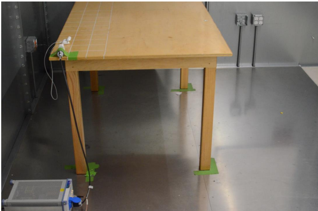
Figure 2: AC Line Conducted Emissions (Side View)
