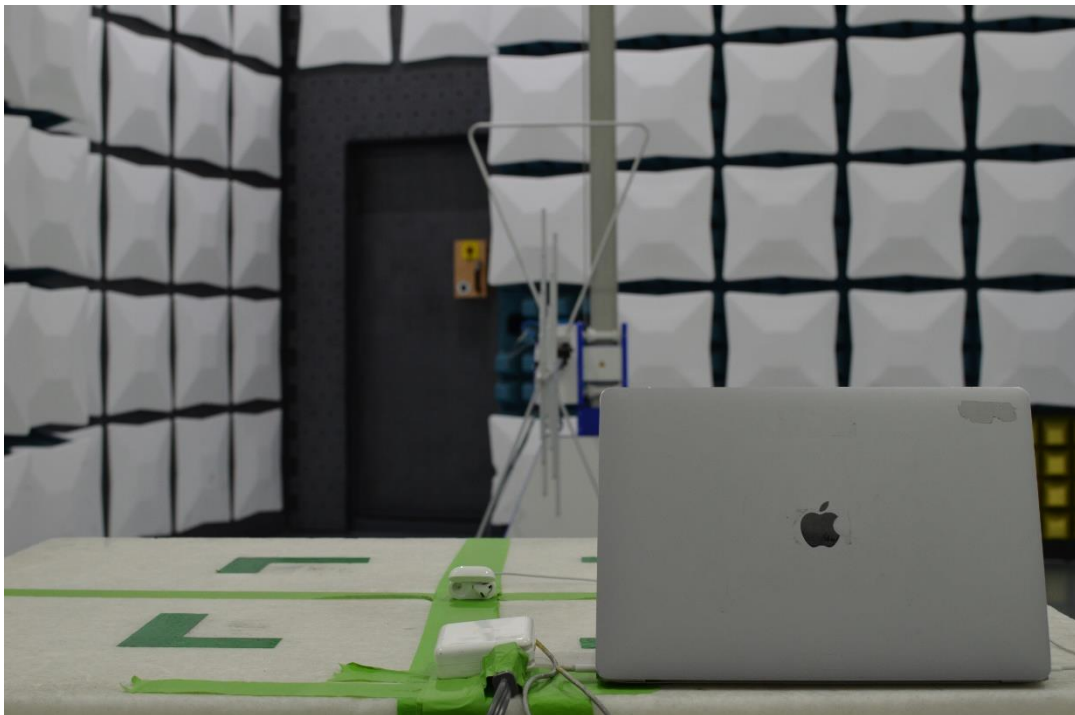
Figure 18: 30MHz-1GHz Test Setup (Rear View)
