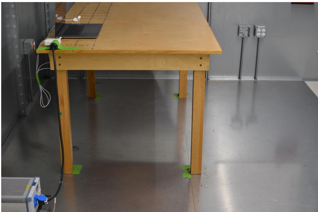
Figure 4: AC Line Conducted Emissions (Side View)
