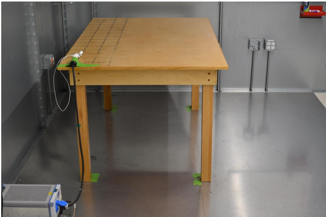
Figure 2: AC Line Conducted Emissions (Side View)
