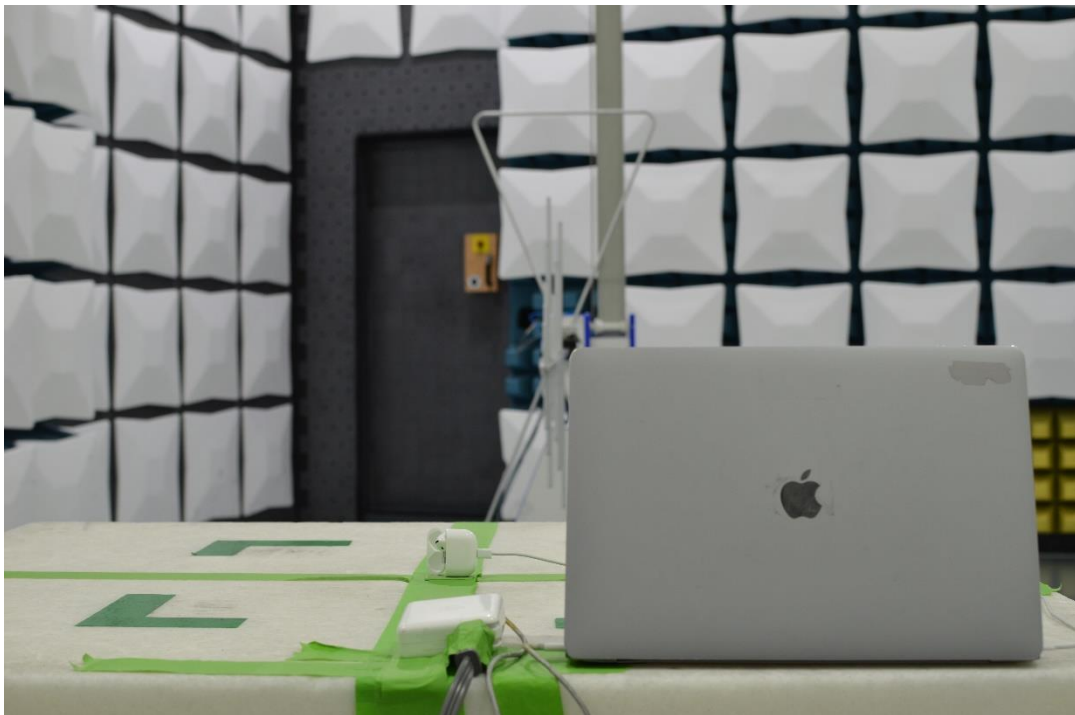
Figure 20: 30MHz-1GHz Test Setup (Rear View)
