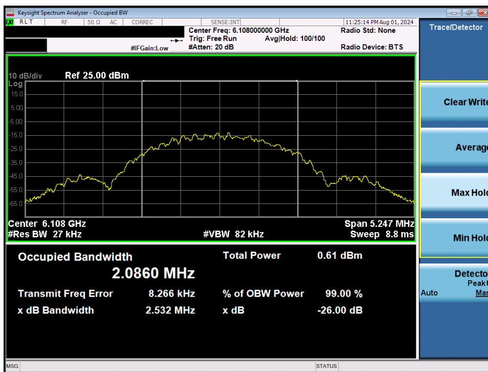
Plot 7-4. 26dB BW & 99% OBW (NB UNII LE, 2Mbps – 6108MHz)
