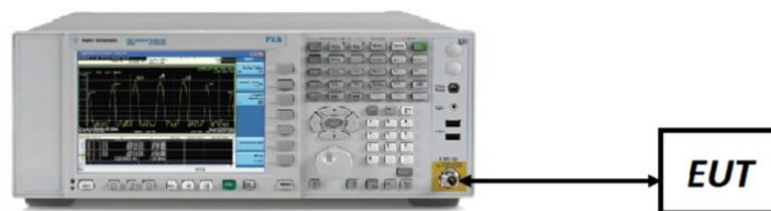
Figure 7-3. Test Instrument & Measurement Setup
