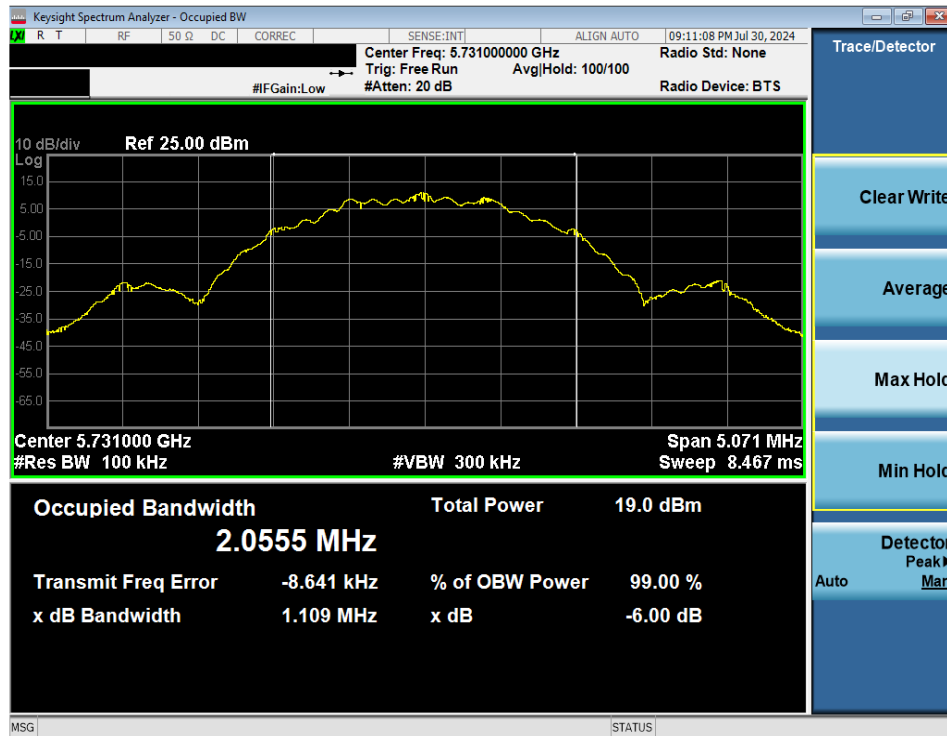
Plot 7-22. 6dB BW & 99% OBW (NB UNII LE2M – 5731MHz)
