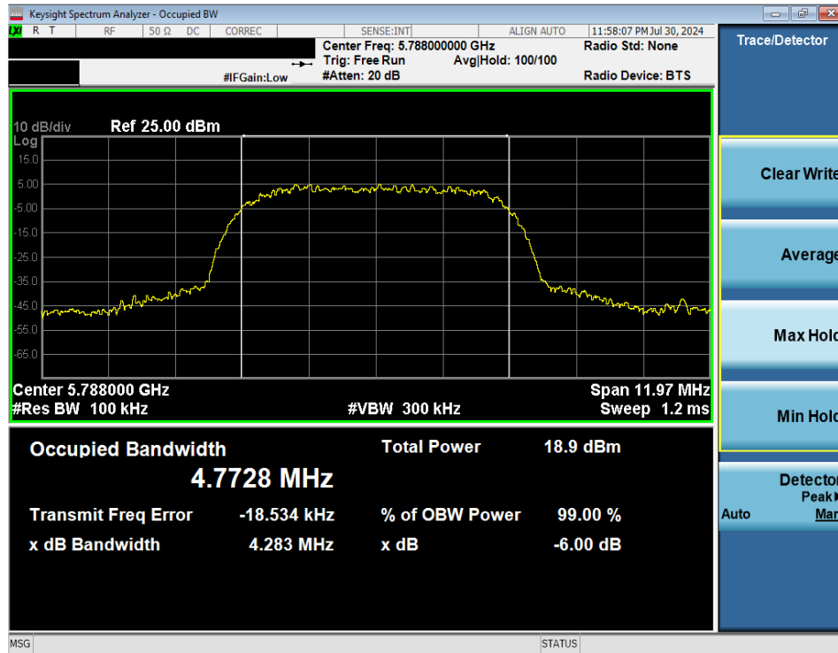
Plot 7-35. 6dB BW & 99% OBW (NB UNII HDRp8 – 5788MHz)
