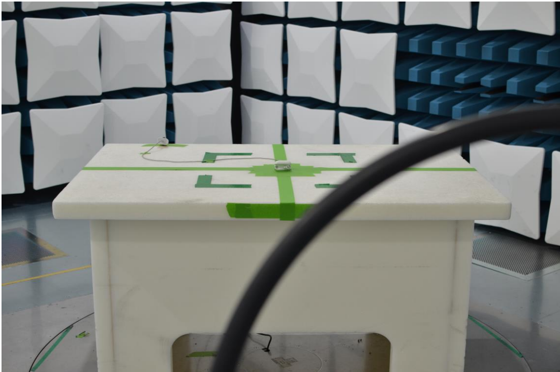
Figure 23: 9kHz-30MHz Test Setup (Front View)
