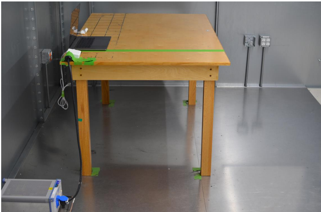
Figure 4: AC Line Conducted Emissions (Side View)
