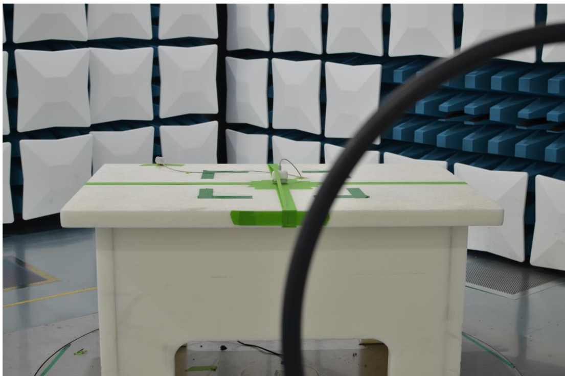
Figure 25: 9kHz-30MHz Test Setup (Front View)
