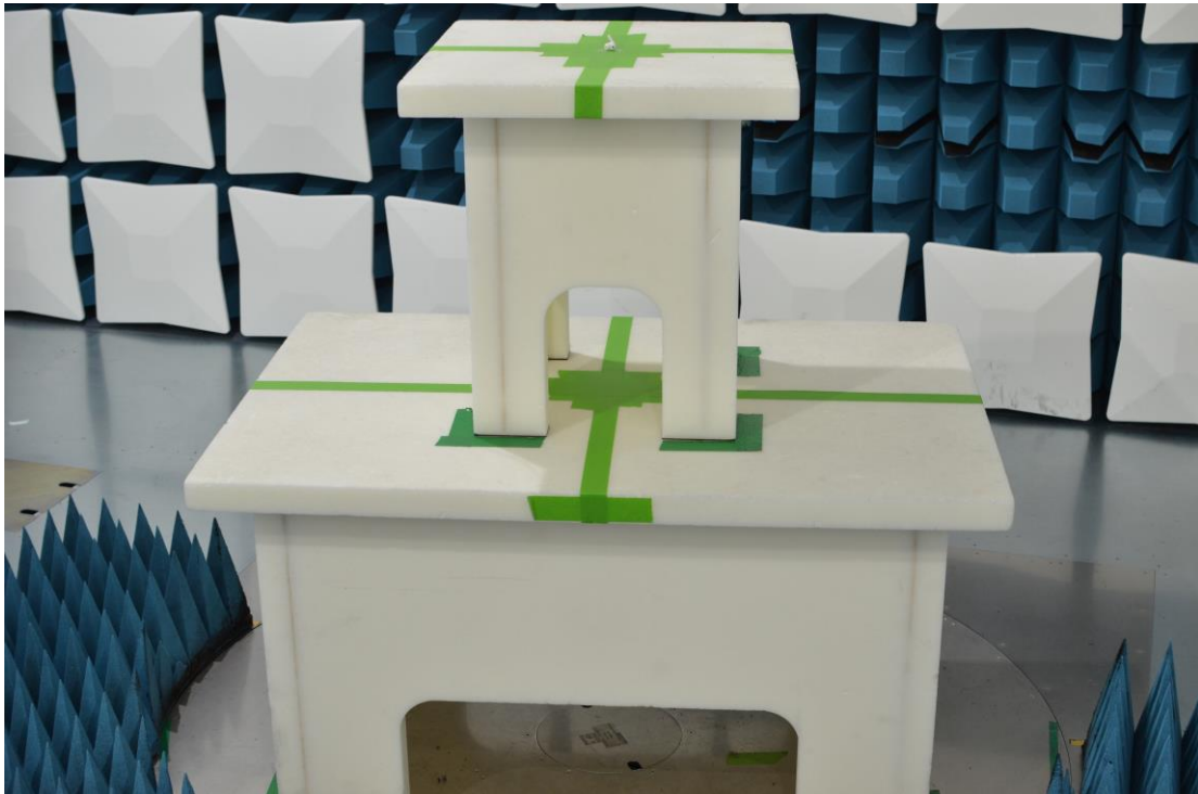
Figure 7: 1-18GHz Test Setup (Front View)
