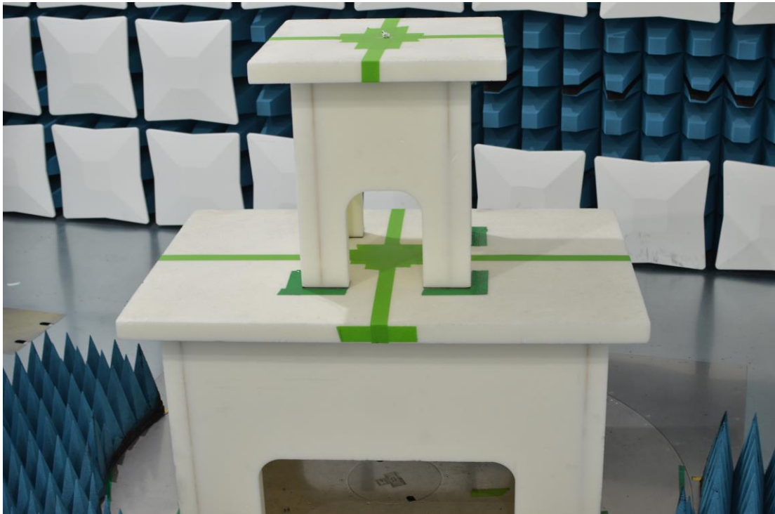
Figure 5: 1-18GHz Test Setup (Front View)
