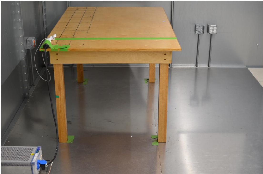
Figure 2: AC Line Conducted Emissions (Side View)
