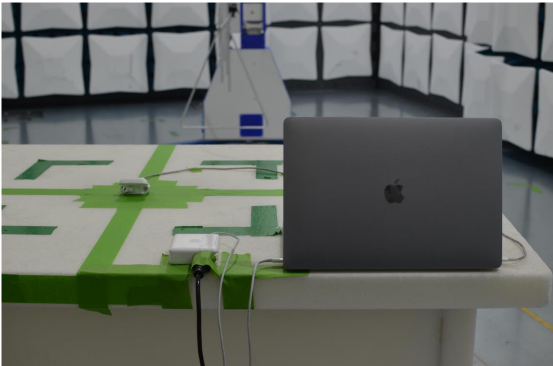
Figure 18: 30MHz-1GHz Test Setup (Rear View)
