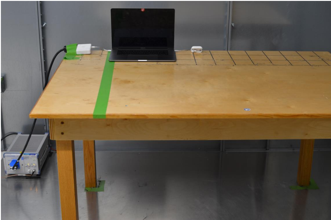
Figure 3: AC Line Conducted Emissions (Front View)
