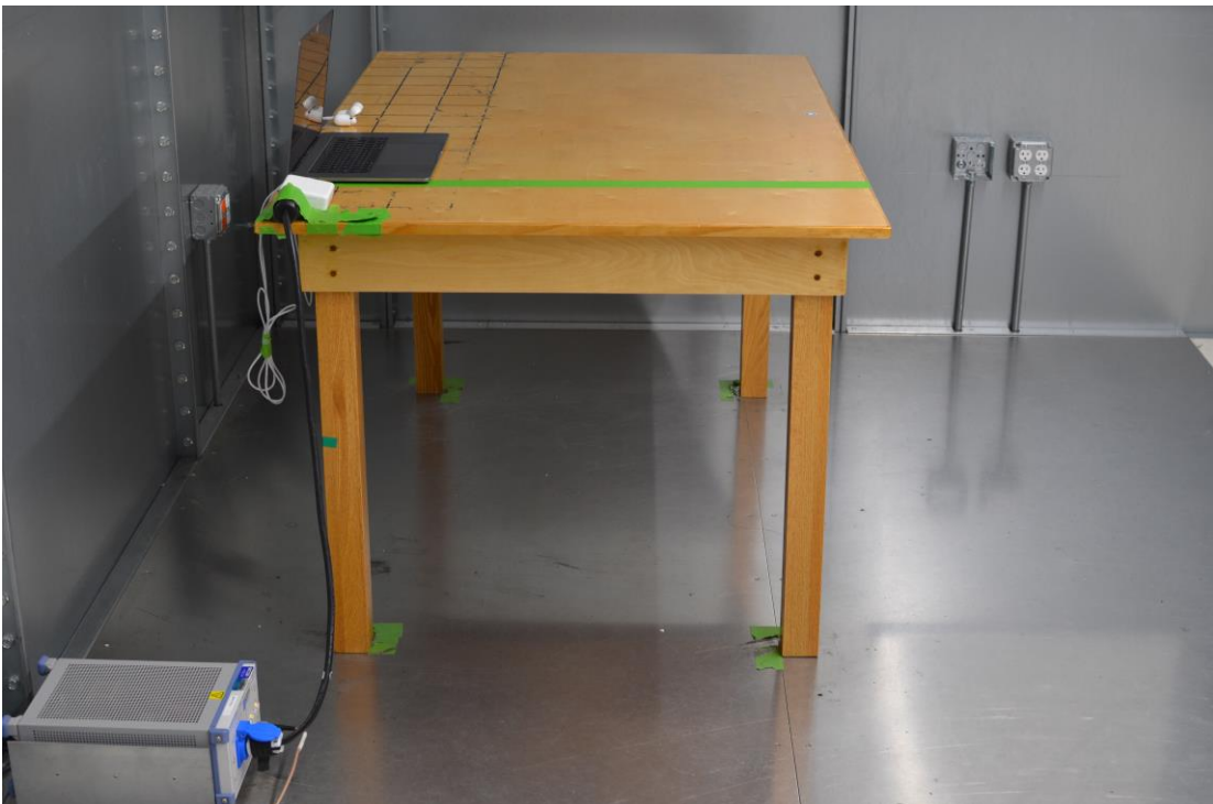
Figure 4: AC Line Conducted Emissions (Side View)
