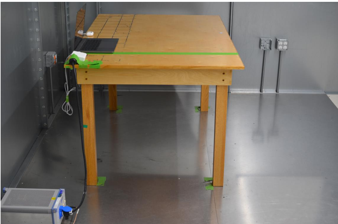
Figure 4: AC Line Conducted Emissions (Side View)
