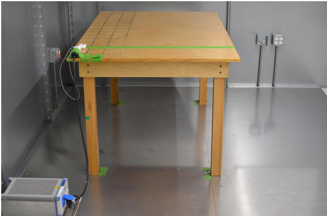
Figure 2: AC Line Conducted Emissions (Side View)
