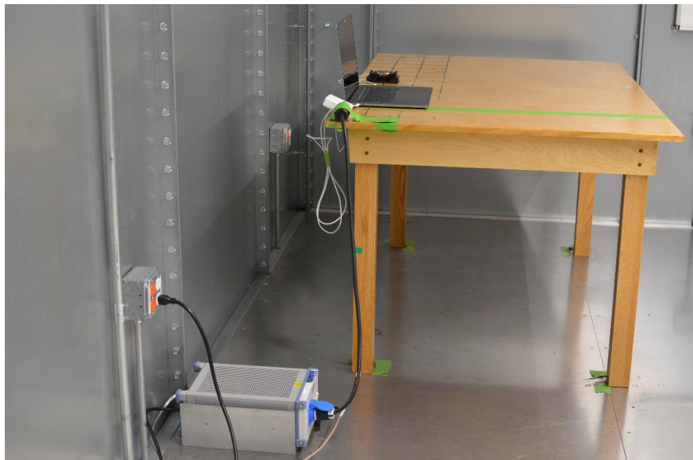
Figure 2: AC Line Conducted Emissions (Side View)
