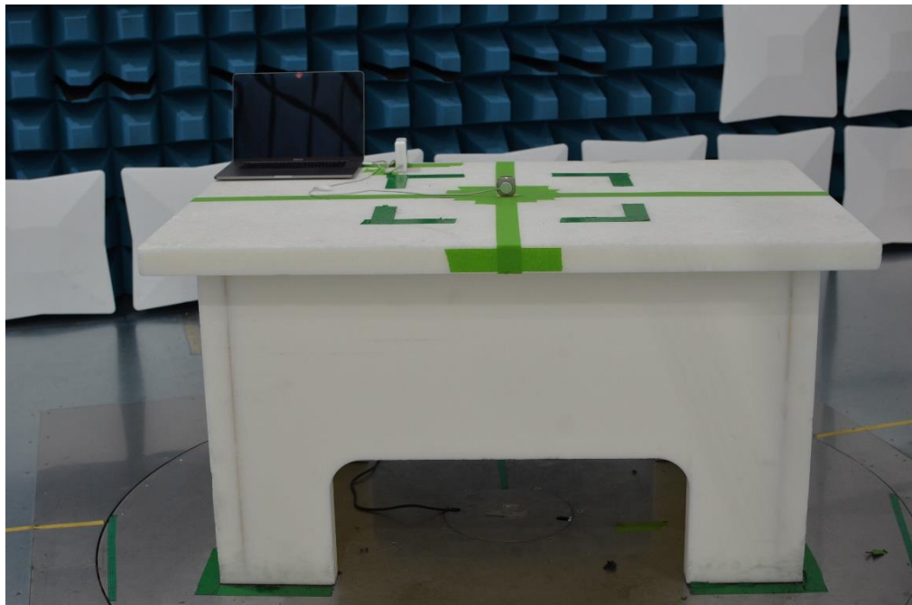
Figure 18: 30MHz-1GHz Test Setup (Front View)
