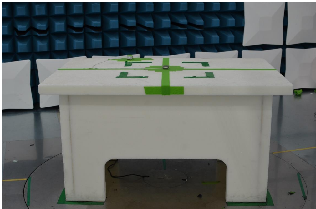
Figure 8: 30MHz-1GHz Test Setup (Front View)
