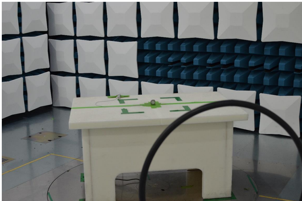
Figure 22: 9kHz-30MHz Test Setup (Front View)
