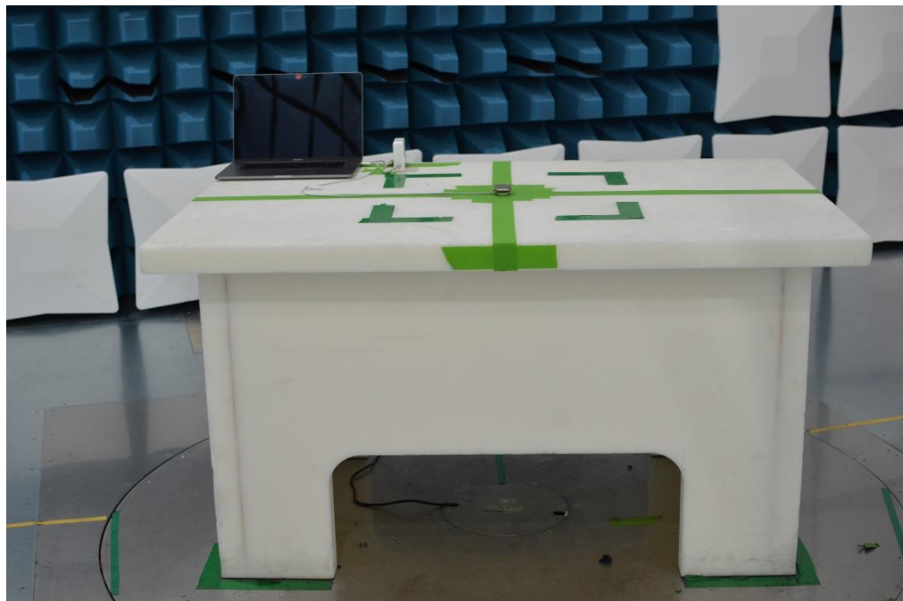
Figure 14: 30MHz-1GHz Test Setup (Front View)
