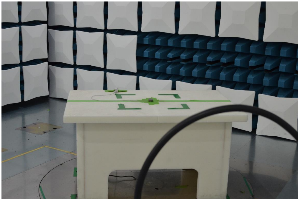
Figure 20: 9kHz-30MHz Test Setup (Front View)
