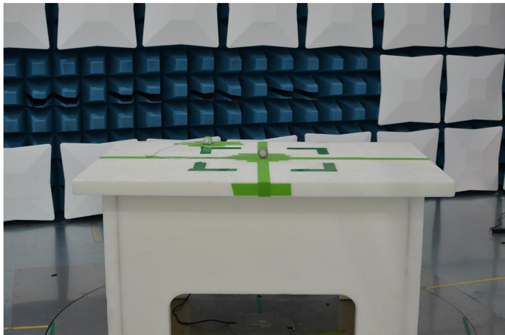
Figure 12: 30MHz-1GHz Test Setup (Front View)
