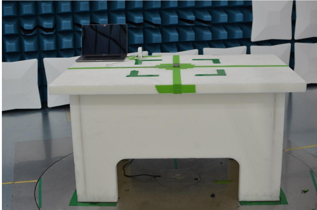
Figure 17: 30MHz-1GHz Test Setup (Front View)
