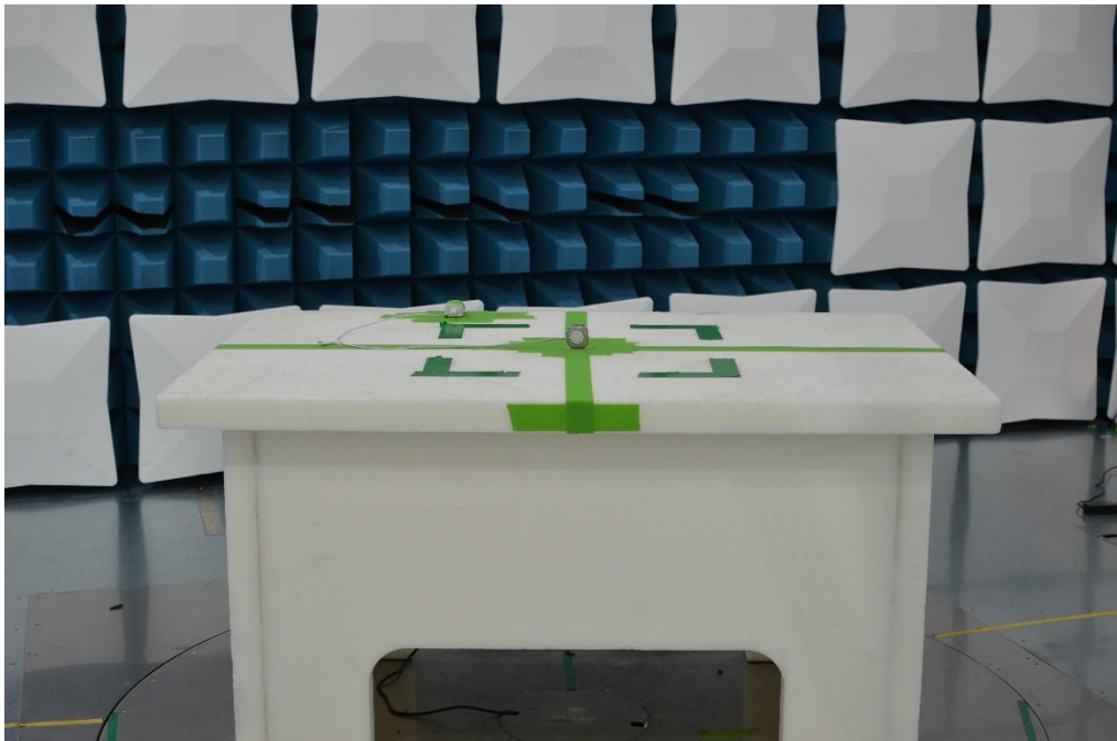
Figure 15: 30MHz-1GHz Test Setup (Front View)
