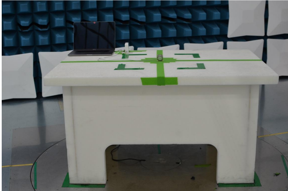
Figure 21: 30MHz-1GHz Test Setup (Front View)
