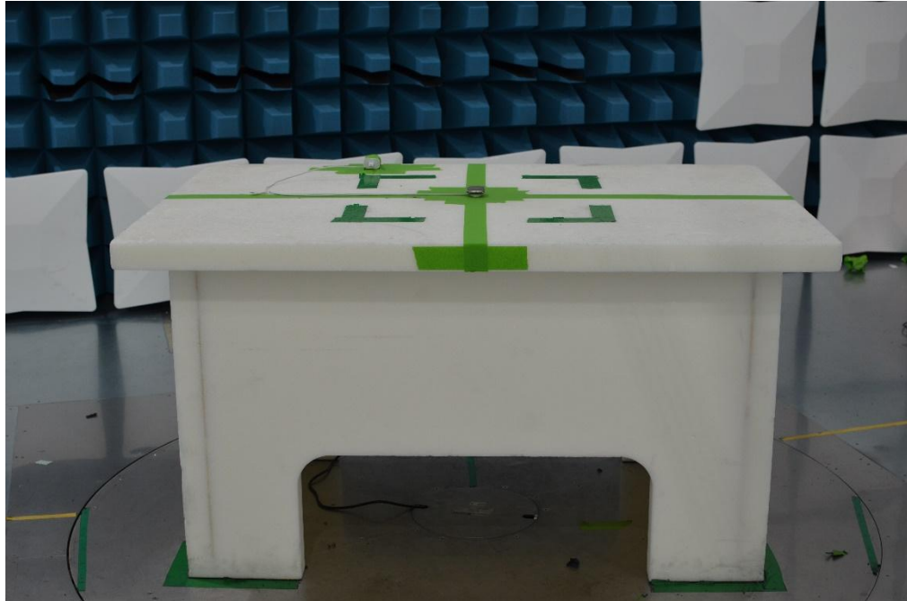
Figure 11: 30MHz-1GHz Test Setup (Front View)
