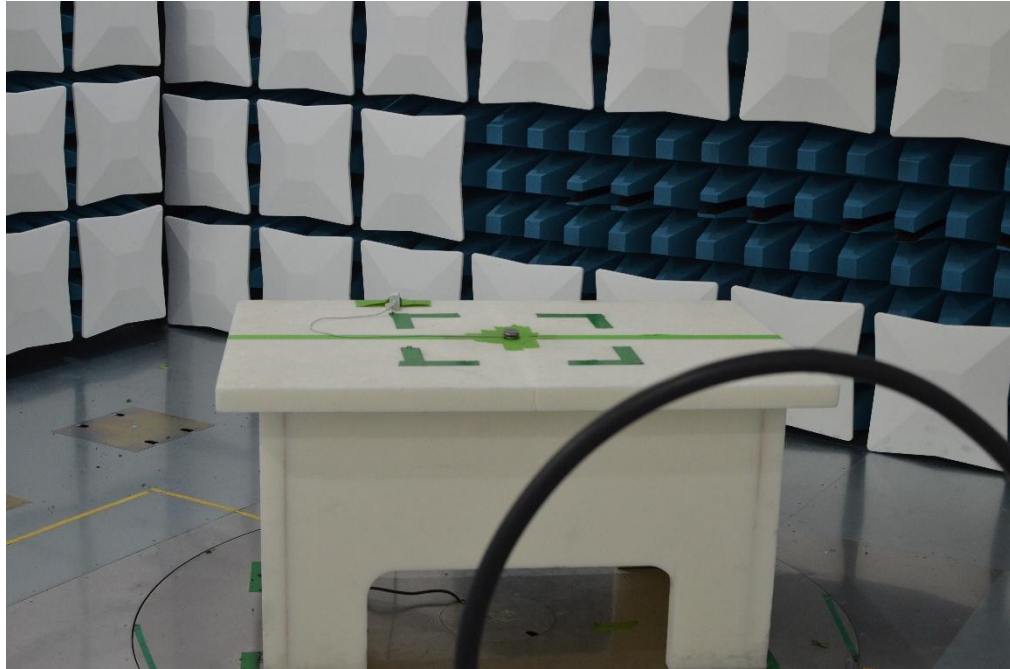
Figure 23: 9kHz-30MHz Test Setup (Front View)
