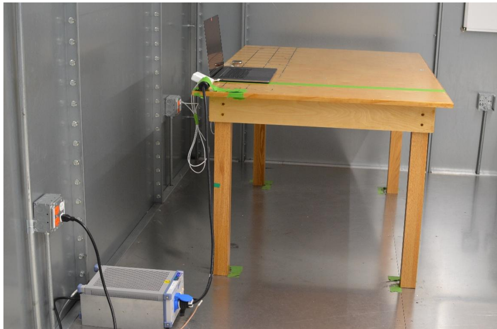
Figure 4: AC Line Conducted Emissions (Side View)
