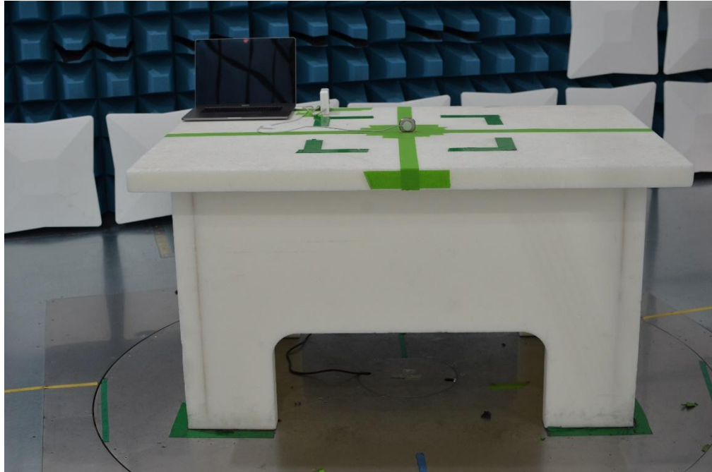
Figure 19: 30MHz-1GHz Test Setup (Front View)
