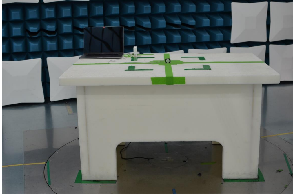
Figure 19: 30MHz-1GHz Test Setup (Front View)
