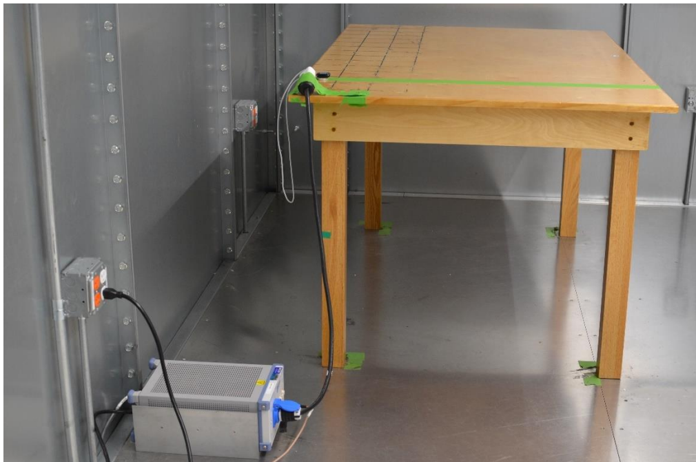
Figure 2: AC Line Conducted Emissions (Side View)
