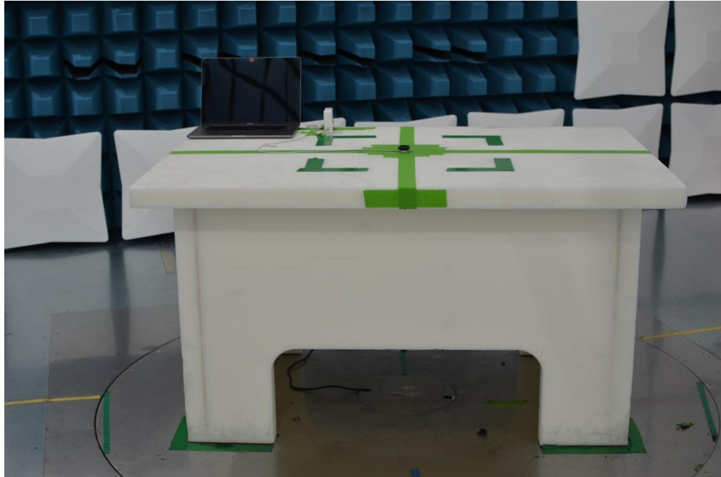
Figure 17: 30MHz-1GHz Test Setup (Front View)
