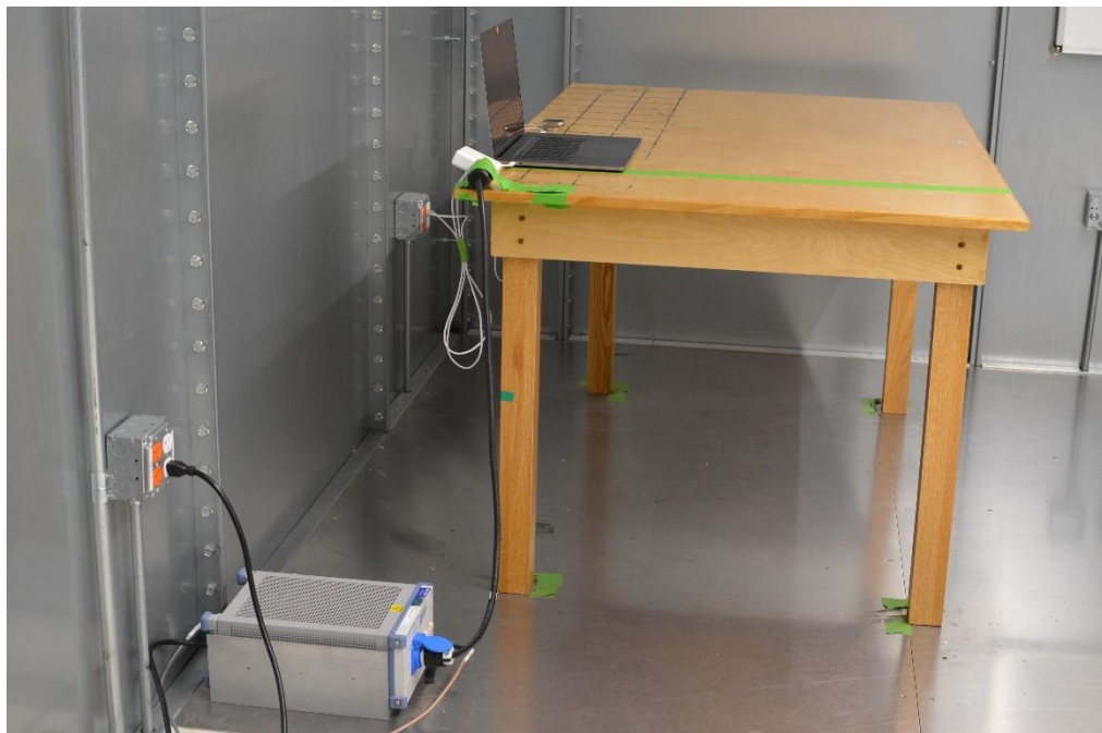
Figure 4: AC Line Conducted Emissions (Side View)
