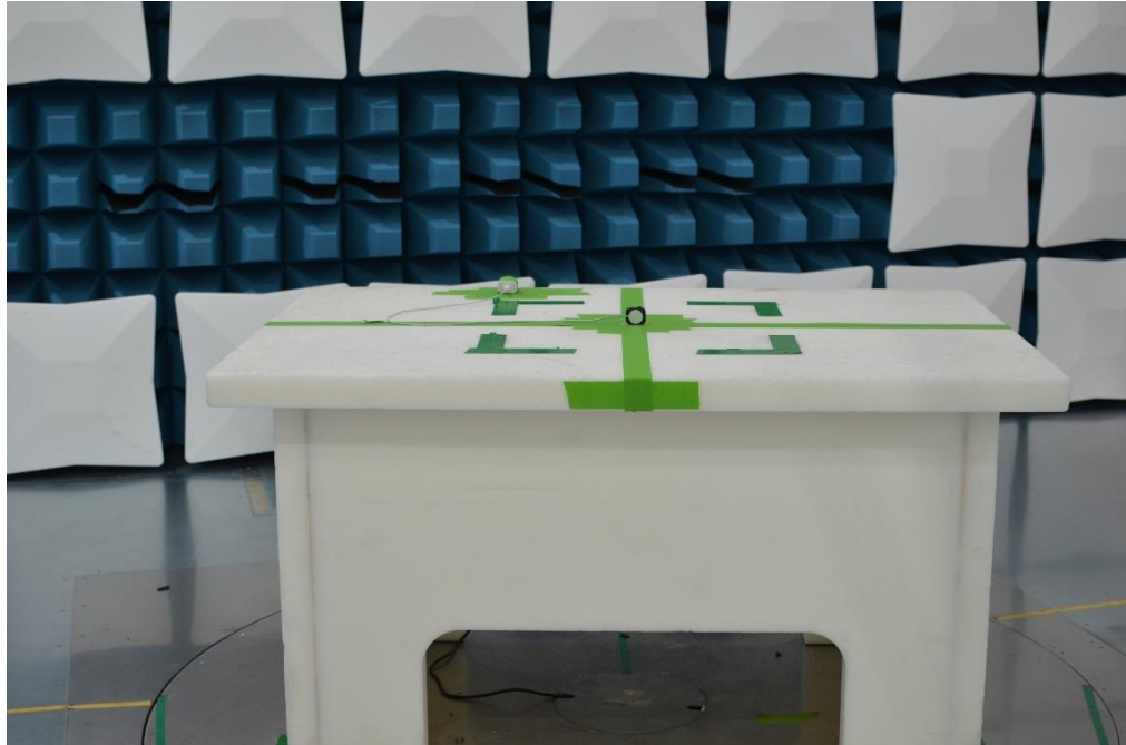
Figure 13: 30MHz-1GHz Test Setup (Front View)
