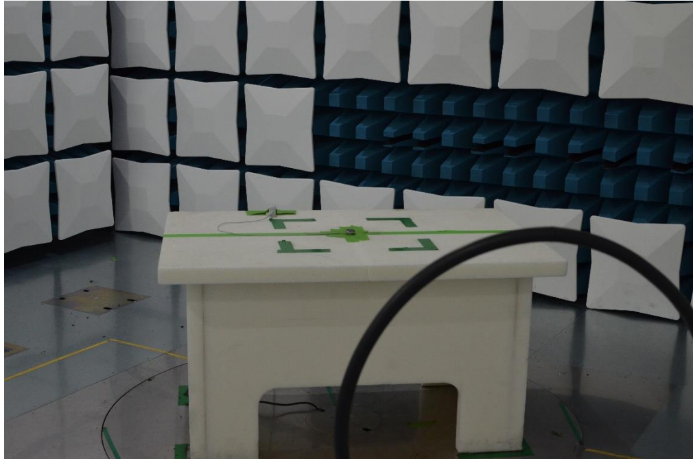
Figure 23: 9kHz-30MHz Test Setup (Front View)
