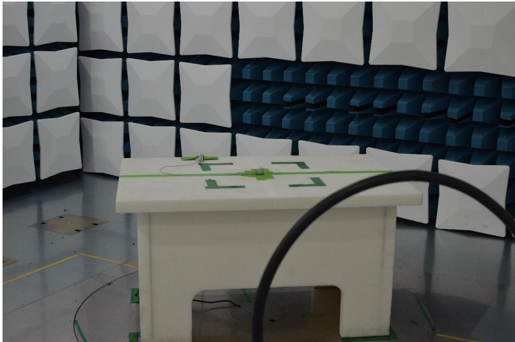
Figure 24: 9kHz-30MHz Test Setup (Front View)
