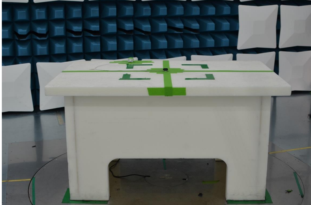
Figure 11: 30MHz-1GHz Test Setup (Front View)
