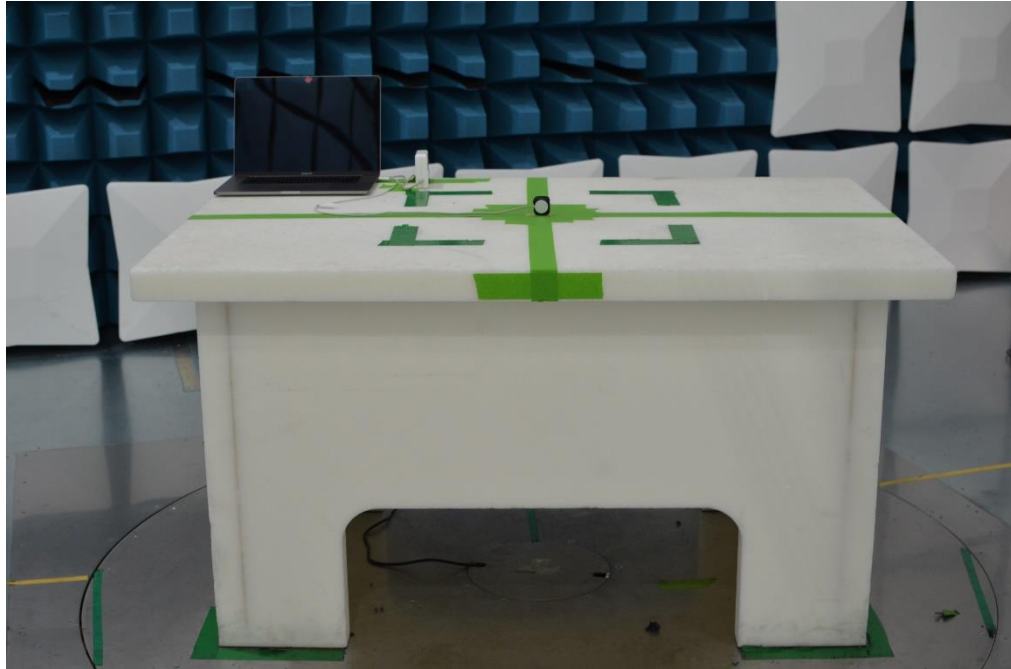
Figure 21: 30MHz-1GHz Test Setup (Front View)
