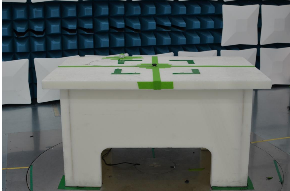
Figure 7: 30MHz-1GHz Test Setup (Front View)
