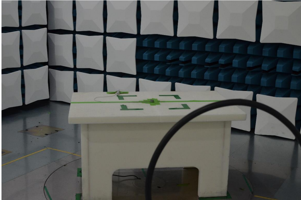
Figure 19: 9kHz-30MHz Test Setup (Front View)
