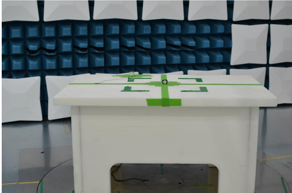
Figure 9: 30MHz-1GHz Test Setup (Front View)
