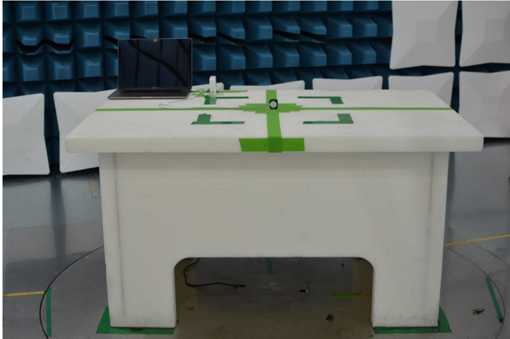
Figure 17: 30MHz-1GHz Test Setup (Front View)
