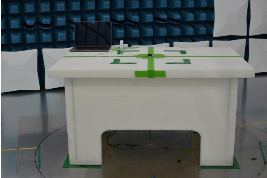
Figure 13: 30MHz-1GHz Test Setup (Front View)
