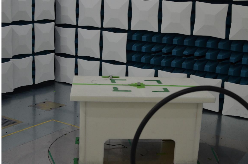
Figure 21: 9kHz-30MHz Test Setup (Front View)
