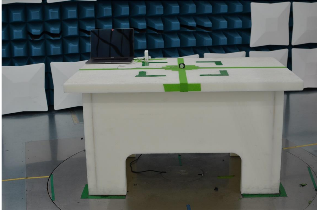
Figure 15: 30MHz-1GHz Test Setup (Front View)
