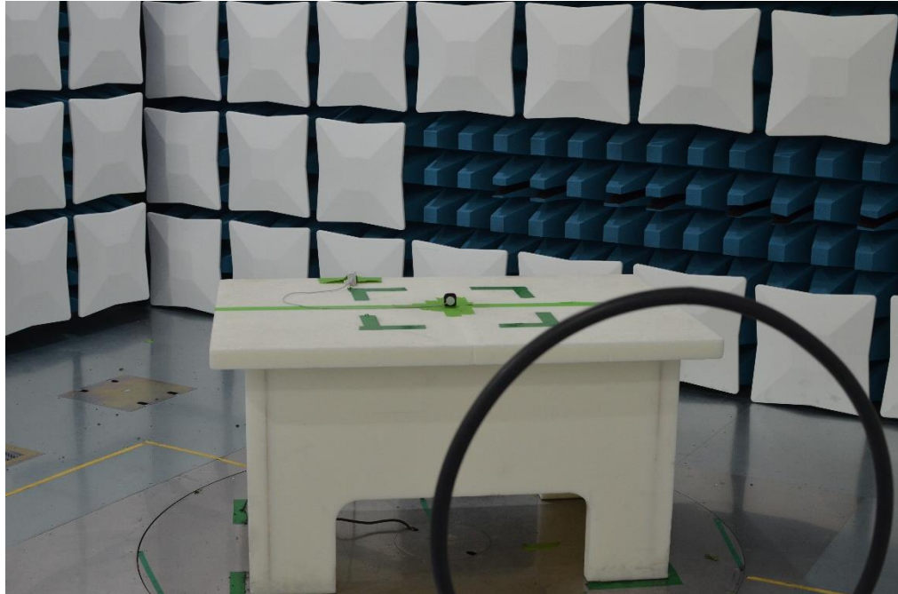
Figure 21: 9kHz-30MHz Test Setup (Front View)
