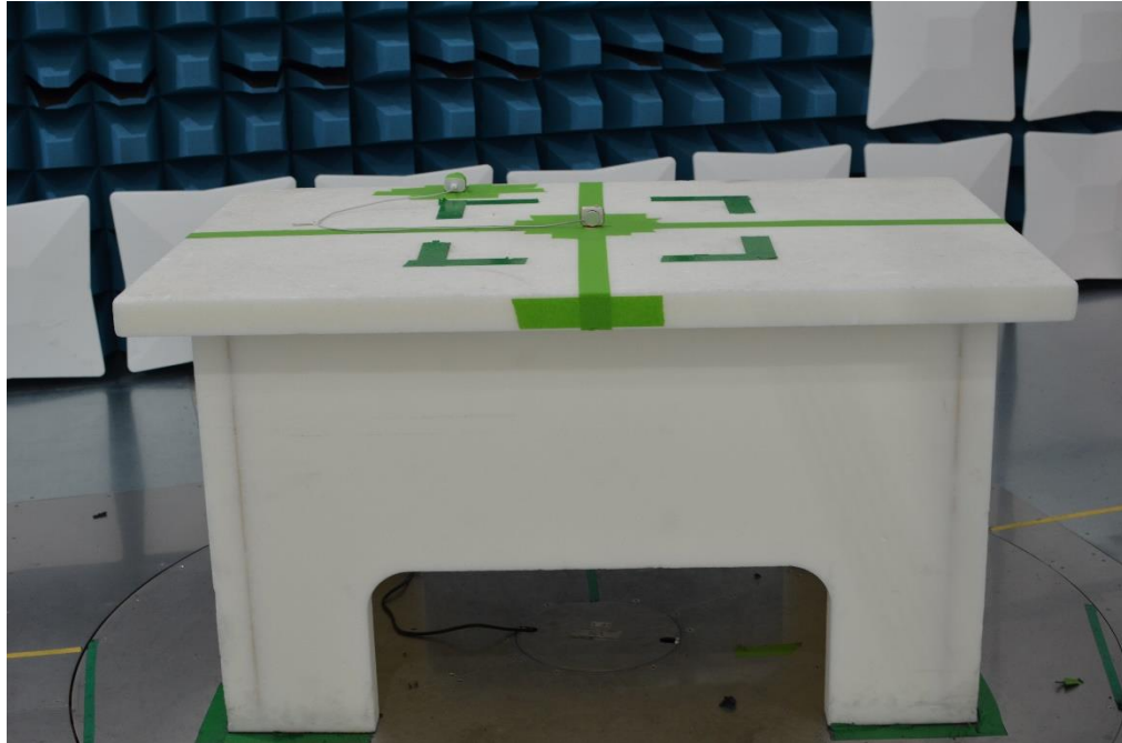
Figure 9: 30MHz-1GHz Test Setup (Front View)
