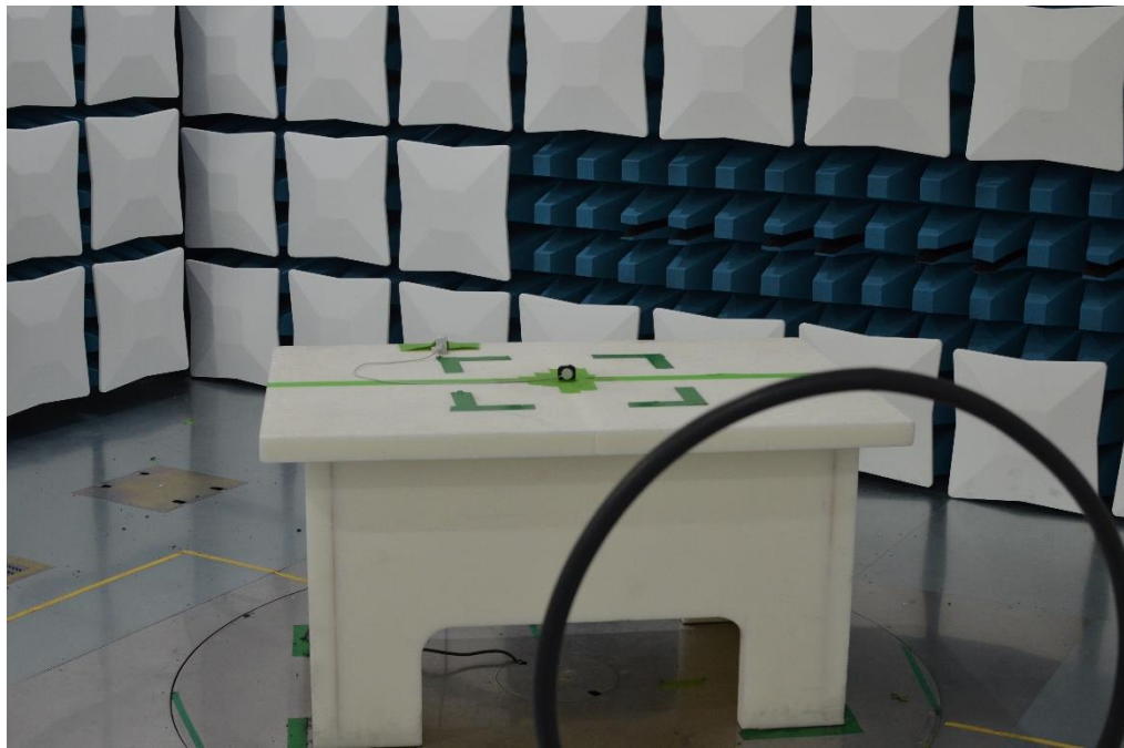
Figure 20: 9kHz-30MHz Test Setup (Front View)
