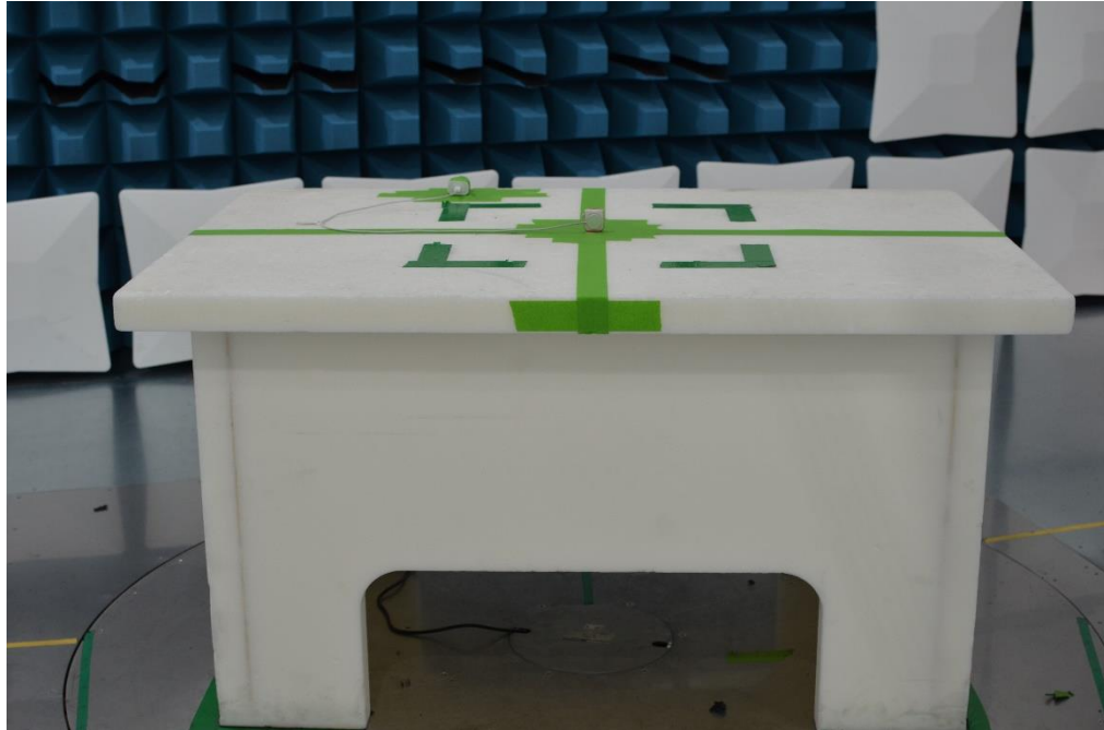
Figure 11: 30MHz-1GHz Test Setup (Front View)
