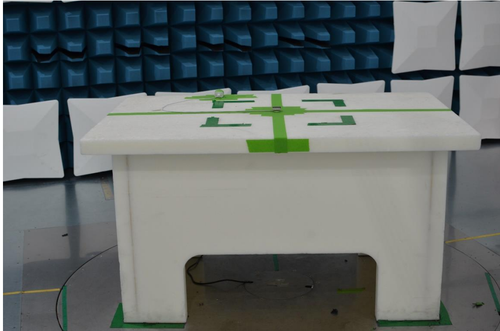
Figure 7: 30MHz-1GHz Test Setup (Front View)
