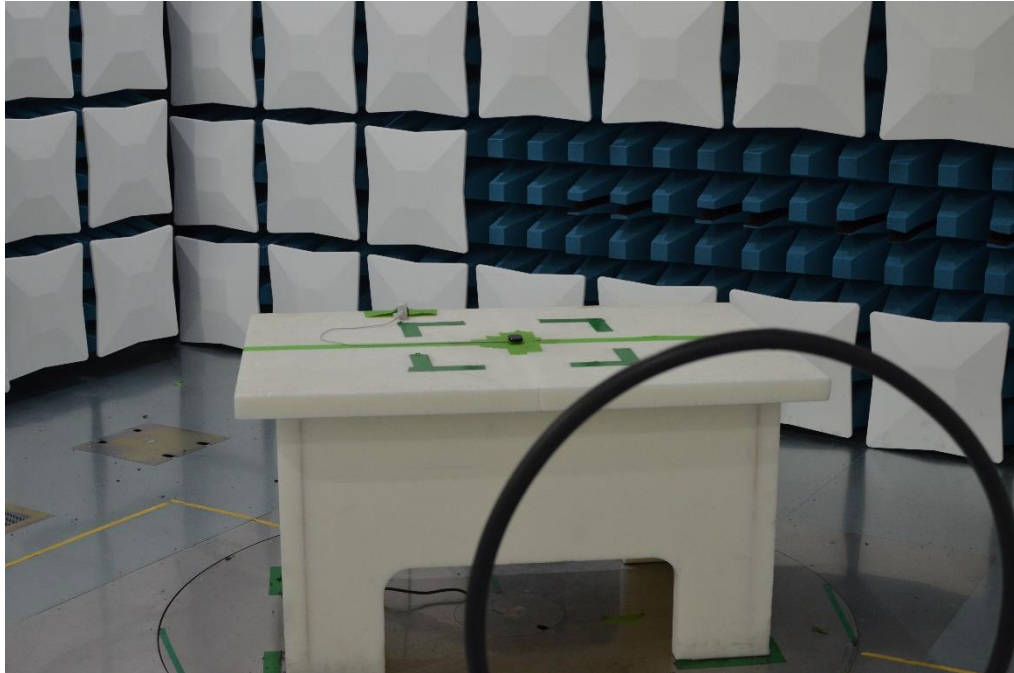
Figure 19: 9kHz-30MHz Test Setup (Front View)
