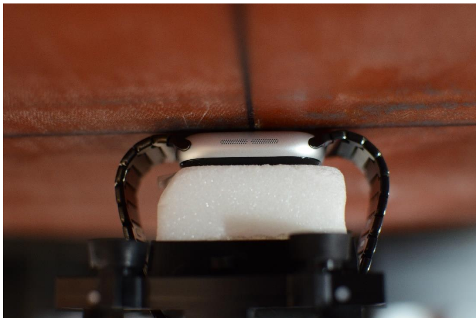
NFC Test Setup Photo 8 – Aluminum with Metal Links Wristband, Extremity, Back Side at 0 mm
