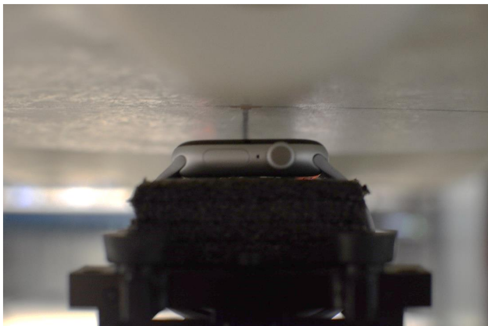
SAR Test Setup Photo 1 – Aluminum with Sport Wristband, Head, Front Side at 10 mm
