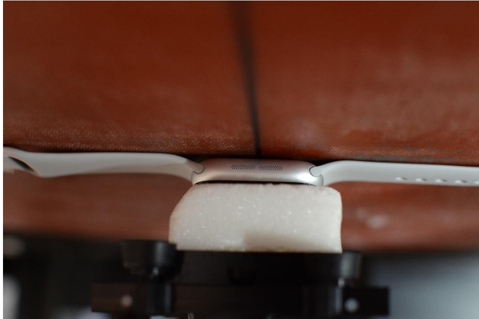
NFC Test Setup Photo 7 – Aluminum with Sport Wristband, Extremity, Back Side at 0 mm
