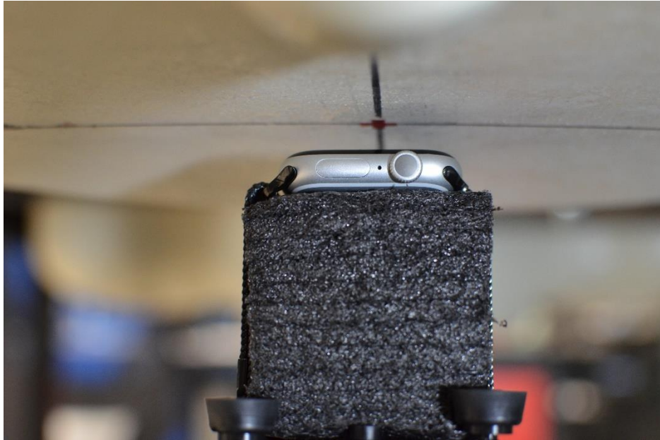
SAR Test Setup Photo 3 – Aluminum with Metal Loop Wristband, Head, Front side at 10mm
