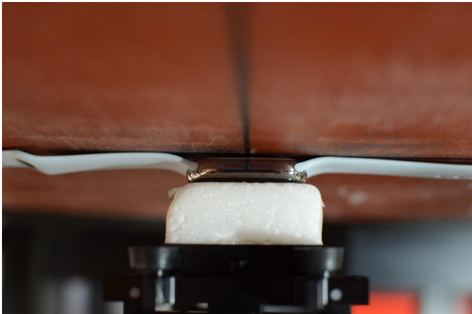
NFC Test Setup Photo 16 – Titanium with Sport Wristband, Extremity, Back side at 0mm
