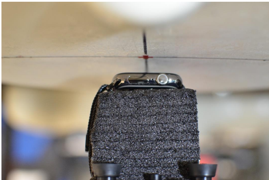
SAR Test Setup Photo 9 – Titanium with Metal Loop Wristband, Head, Front side at 10mm
