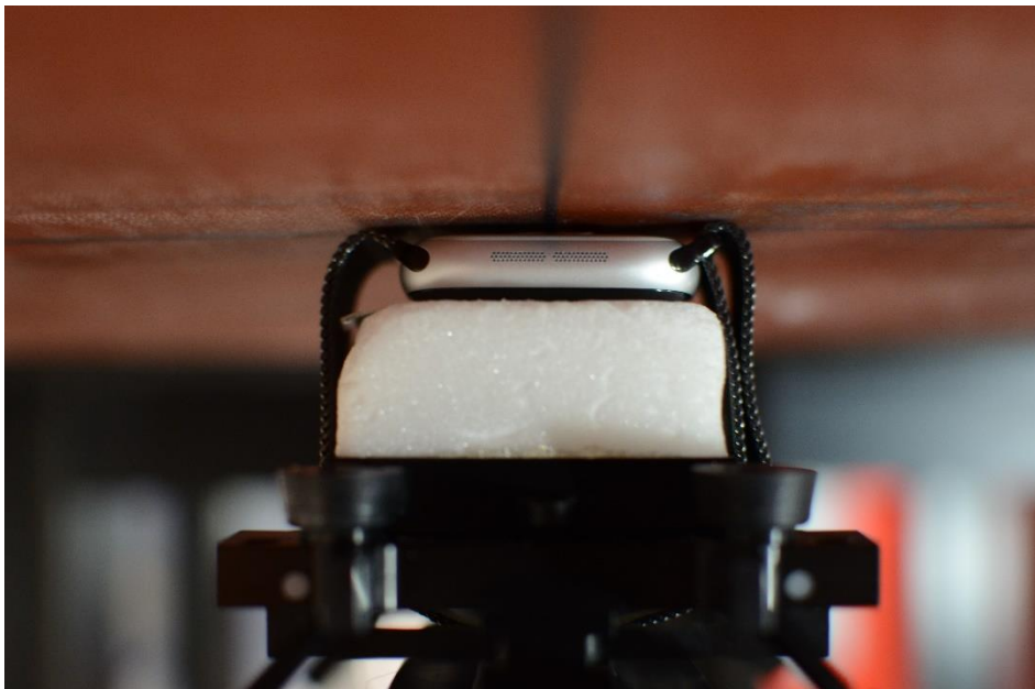
NFC Test Setup Photo 15 – Aluminum with Metal Loop Wristband, Extremity, Back side at 0mm
