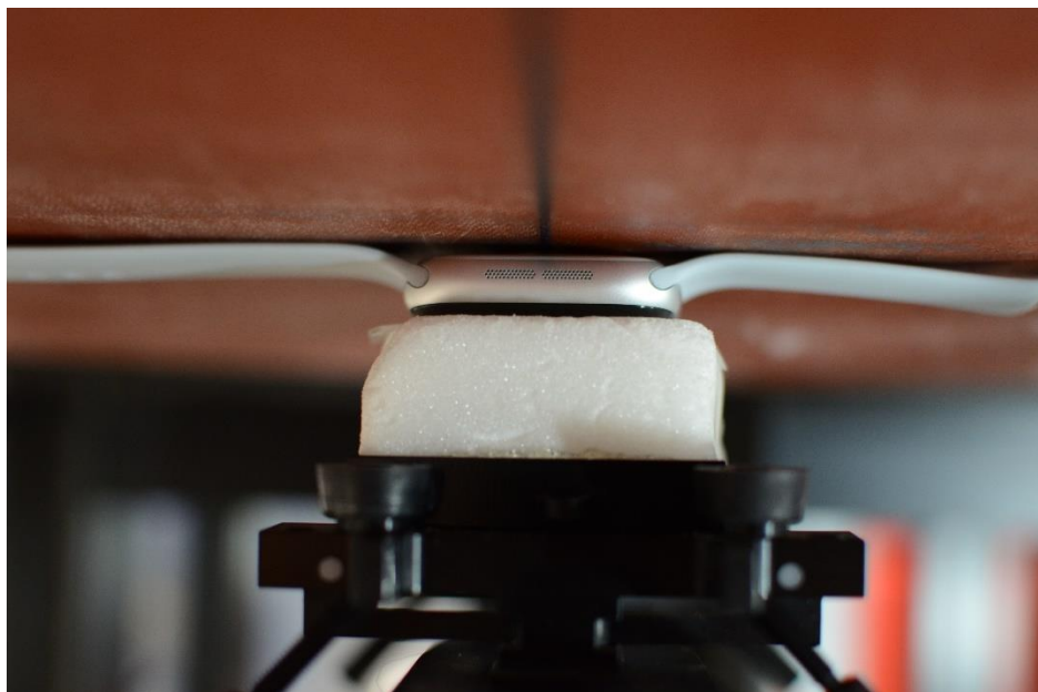
NFC Test Setup Photo 13 – Aluminum with Sport Wristband, Extremity, Back side at 0mm
