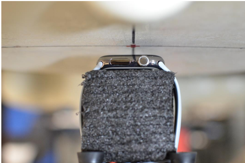
SAR Test Setup Photo 7 – Titanium with Sport Wristband, Head, Front side at 10mm
