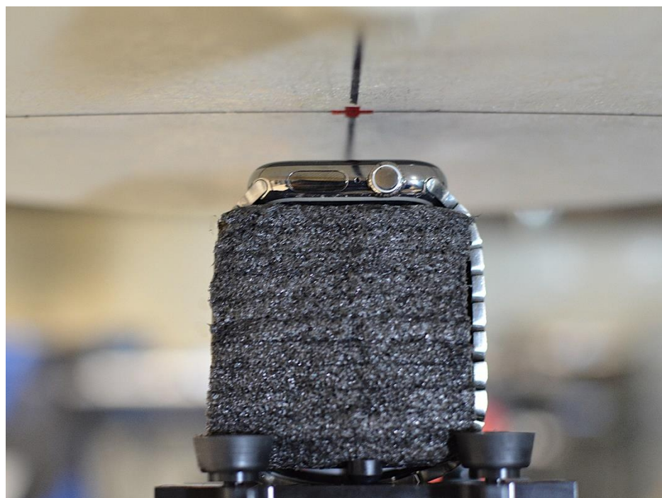
SAR Test Setup Photo 8 – Titanium with Metal Links Wristband, Head, Front side at 10mm
