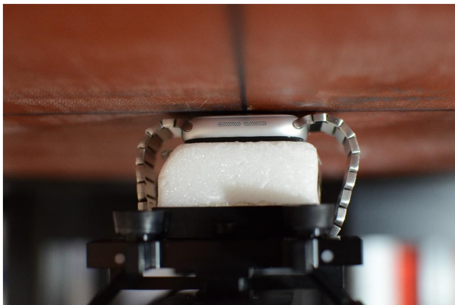
NFC Test Setup Photo 14 – Aluminum with Metal Links Wristband, Extremity, Back side at 0mm
