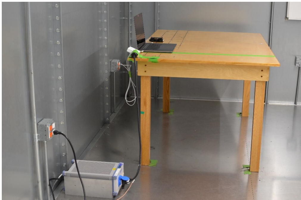
Figure 2: AC Line Conducted Emissions (Side View)
