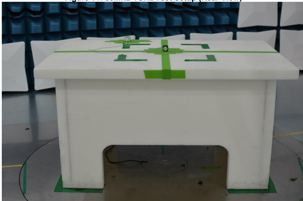
Figure 12: 30MHz-1GHz Test Setup (Front View)
