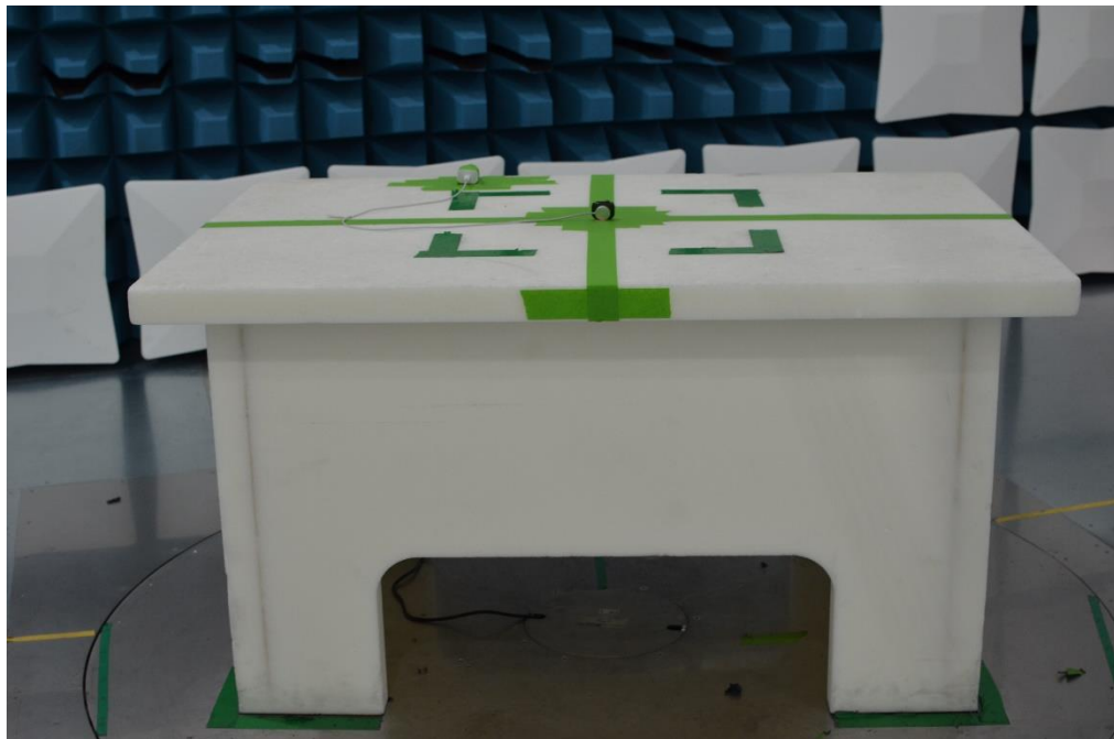
Figure 10: 30MHz-1GHz Test Setup (Front View)
