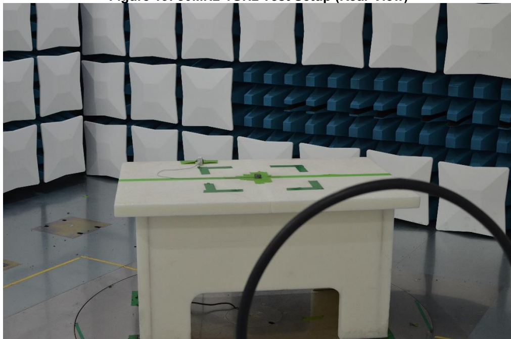
Figure 20: 9kHz-30MHz Test Setup (Front View)
