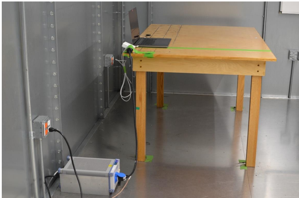
Figure 4: AC Line Conducted Emissions (Side View)
