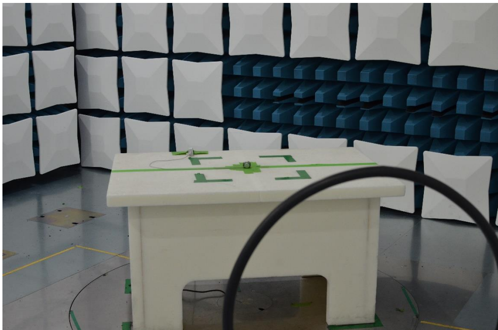
Figure 21: 9kHz-30MHz Test Setup (Front View)
