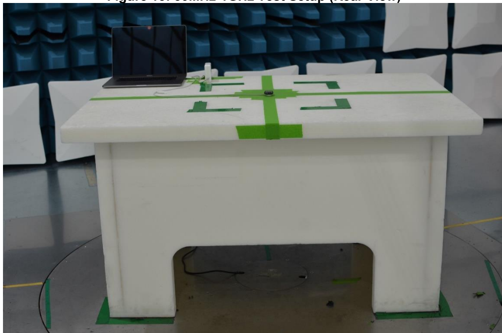
Figure 14: 30MHz-1GHz Test Setup (Front View)
