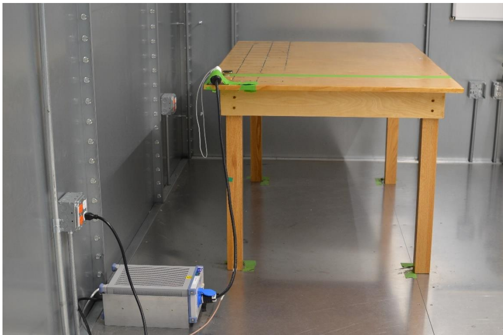
Figure 2: AC Line Conducted Emissions (Side View)
