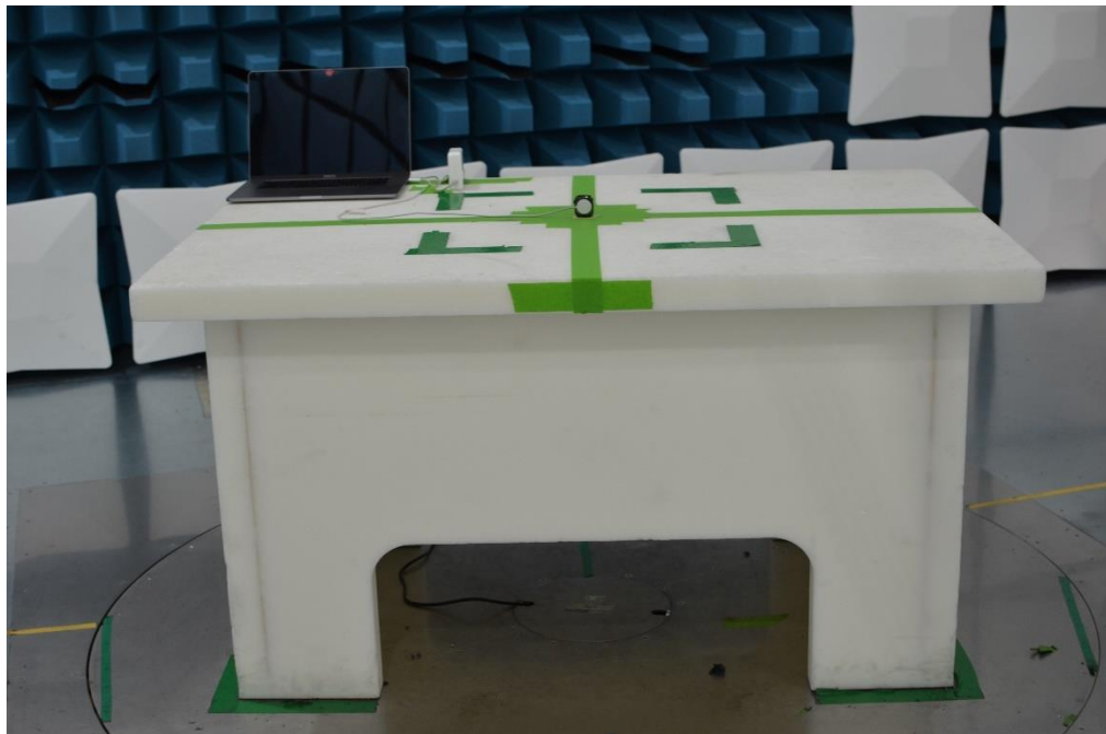
Figure 18: 30MHz-1GHz Test Setup (Front View)
