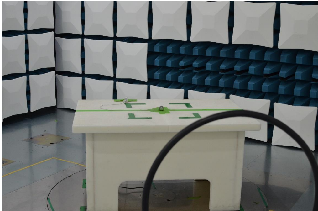
Figure 22: 9kHz-30MHz Test Setup (Front View)
