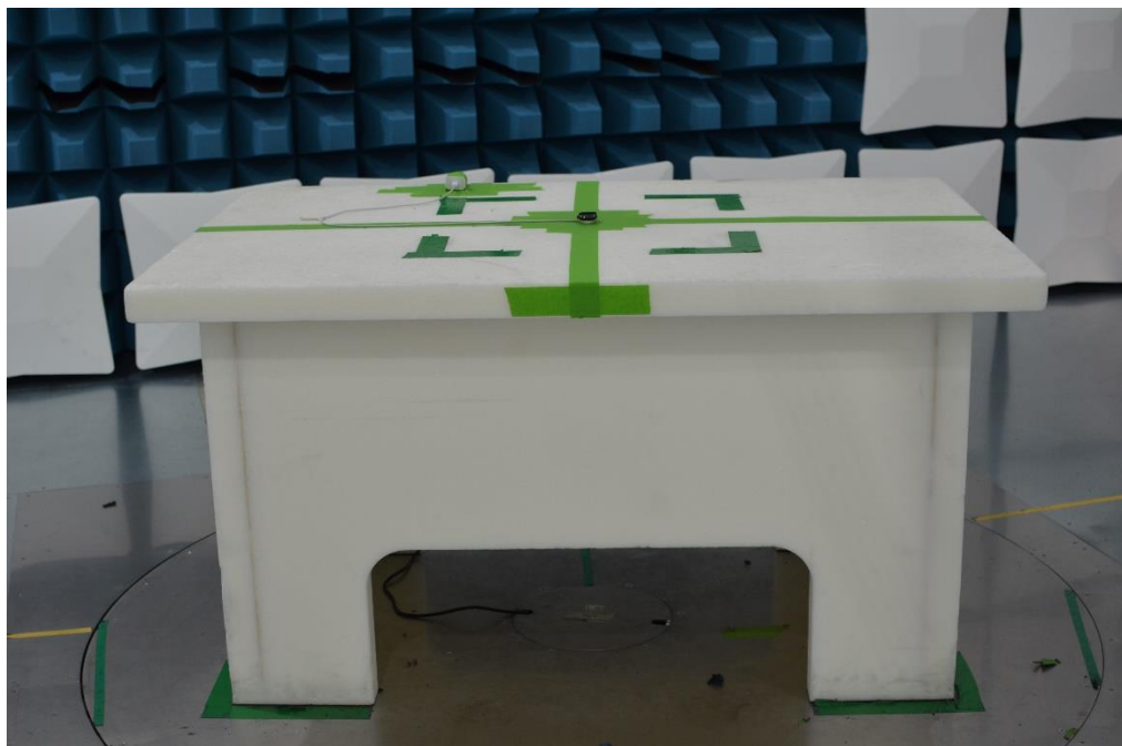
Figure 8: 30MHz-1GHz Test Setup (Front View)
