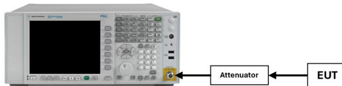
Figure 7-3. Test Instrument & Measurement Setup
