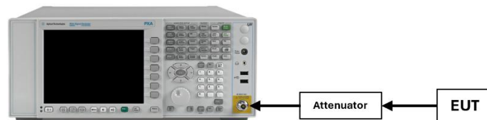
Figure 7-5. Test Instrument & Measurement Setup
