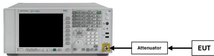
Figure 7-1. Test Instrument & Measurement Setup
