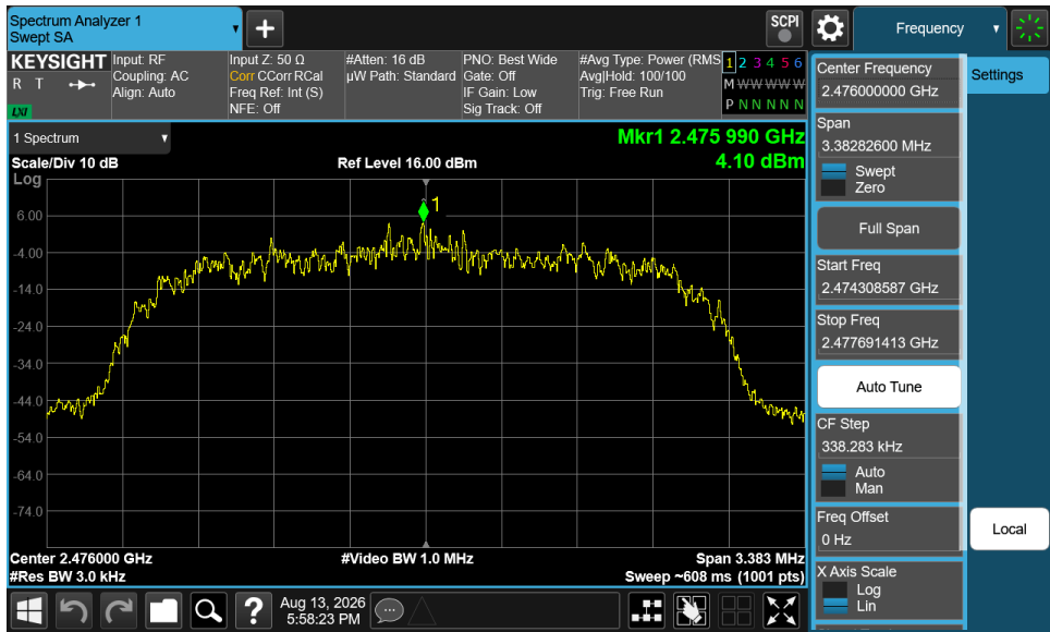
Plot 7-27. Power Spectral Density Plot (Bluetooth (HDR4), 4Mbps, – Ch. 73)
