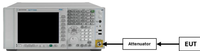
Figure 7-6. Test Instrument & Measurement Setup
