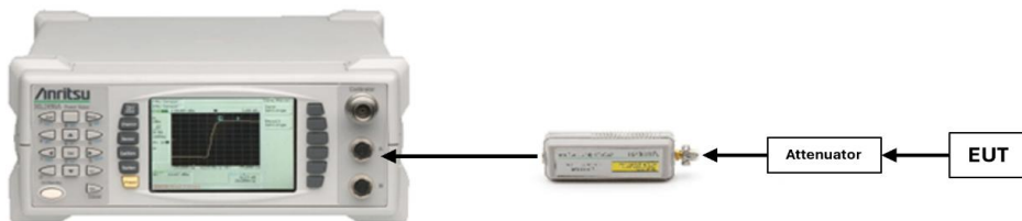
Figure 7-2. Test Instrument & Measurement Setup for Peak and Average Power Measurement
