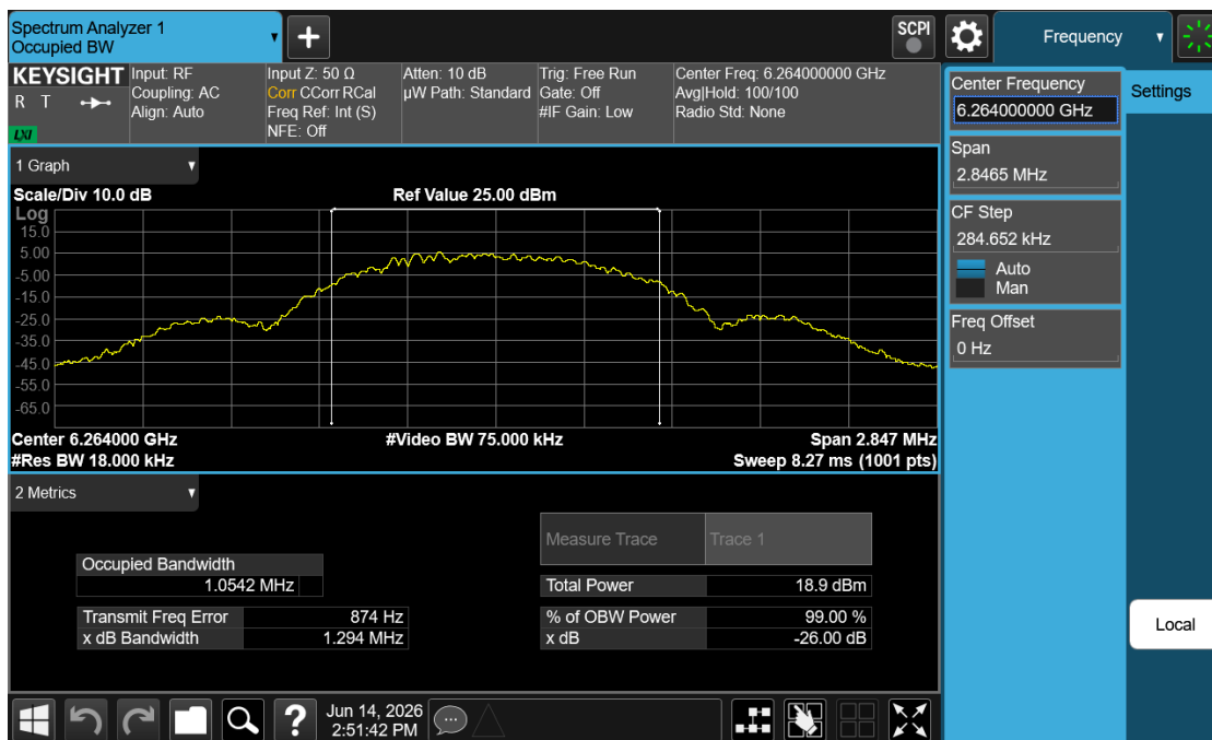
Plot 7-2. 26dB BW & 99% OBW (NB UNII LE1M – 6264MHz)
