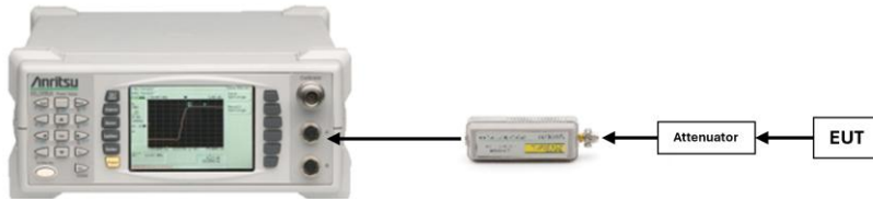
Figure 7-2. Test Instrument & Measurement Setup
