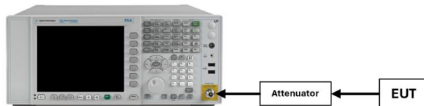
Figure 7-3. Test Instrument & Measurement Setup
