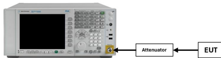
Figure 7-1. Test Instrument & Measurement Setup
