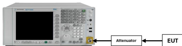
Figure 7-4. Test Instrument & Measurement Setup
