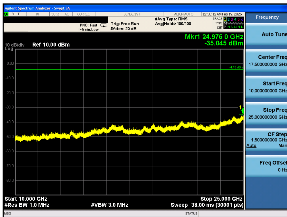
Plot 7-24. Conducted Spurious Plot (Bluetooth, GFSK – Ch. 0)
