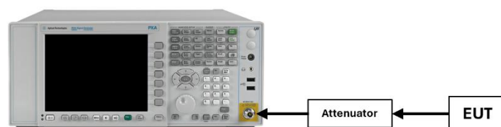
Figure 7-5. Test Instrument & Measurement Setup
