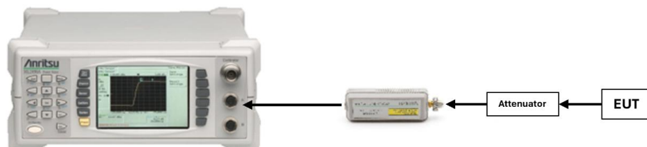
Figure 7-2. Test Instrument & Measurement Setup for Peak and Average Power Measurement
