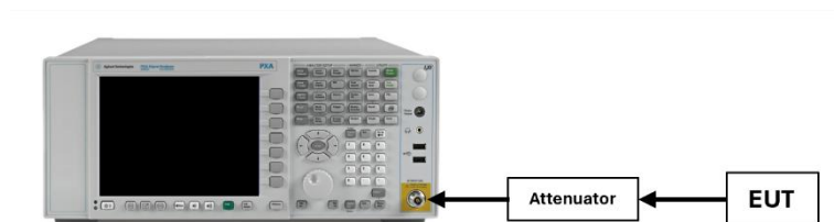
Figure 7-2. Test Instrument & Measurement Setup
