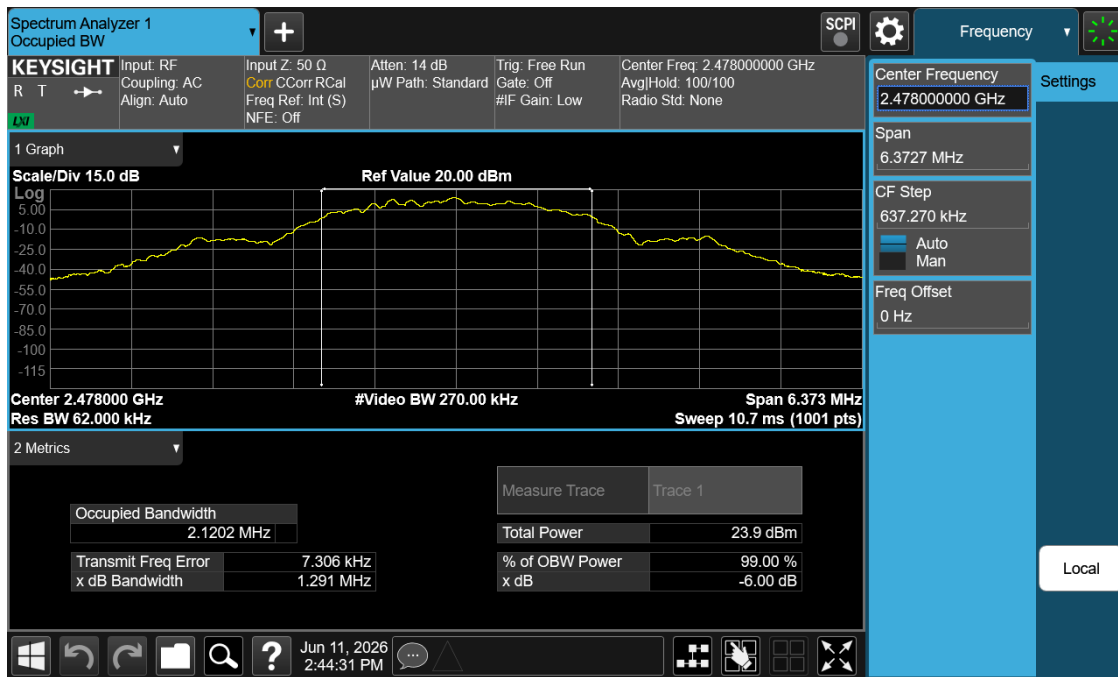
Plot 7-6. 99% OBW Plot (Bluetooth (LE), 2Mbps– Ch. 36)
