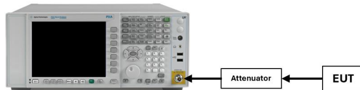
Figure 7-5. Test Instrument & Measurement Setup
