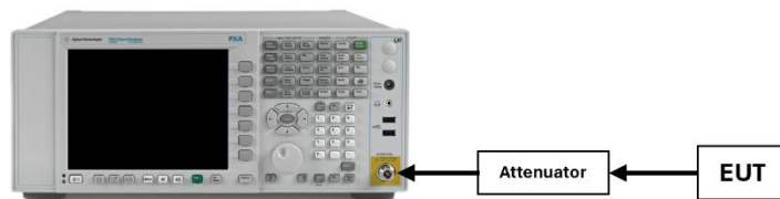
Figure 7-2. Test Instrument & Measurement Setup
