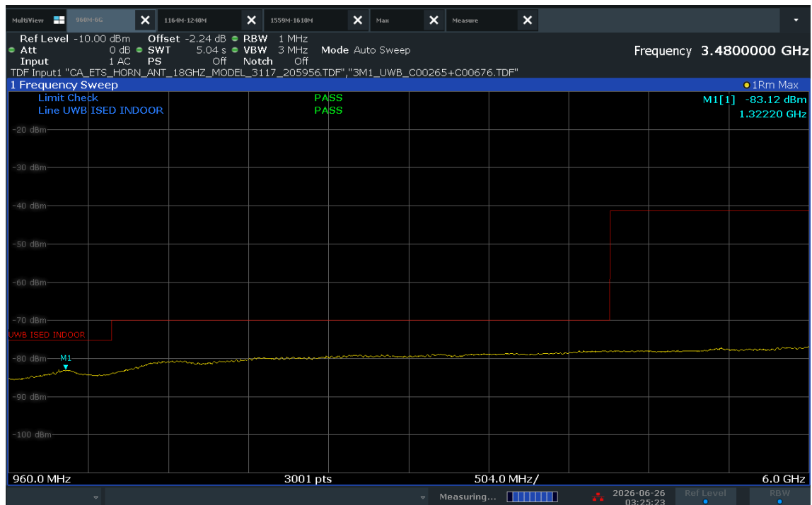
Plot 7-26. ISD Radiated Spurious Emission 960-6000MHz (Ch.9, Config 9, Payload 125B Ant. Pol. V)
