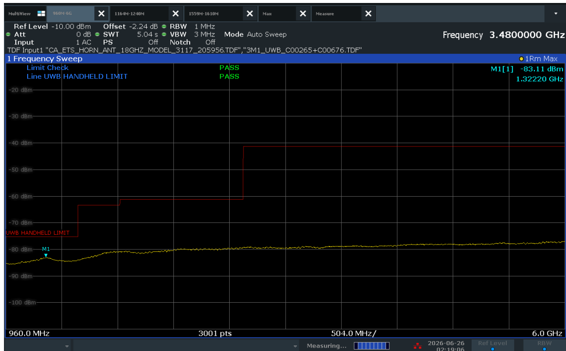
Plot 7-15. FCC Radiated Spurious Emission 960-6000MHz (Ch. 5, Config 9, Payload 125B Ant. Pol. H)
