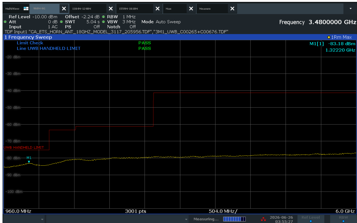
Plot 7-23. FCC Radiated Spurious Emission 960-6000MHz (Ch. 9, Config 9, Payload 125B Ant. Pol. H)
