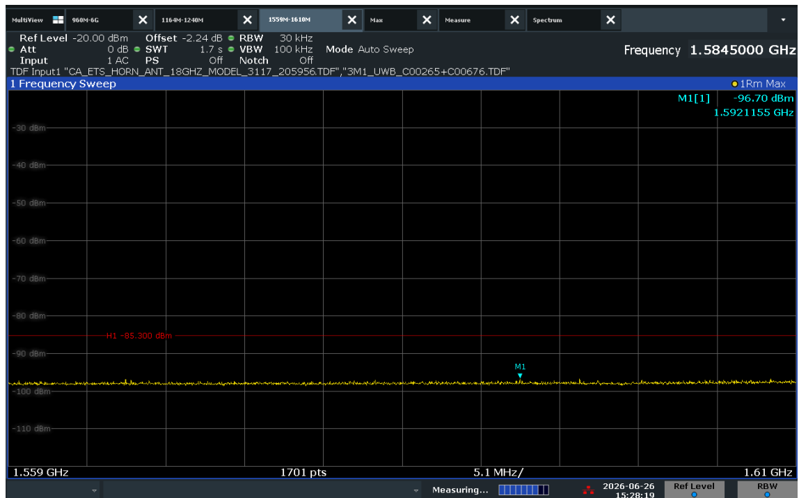
Plot 7-20. Radiated Spurious Emission 1559-1610MHz (Ch. 5, Config 9, Payload 125B Ant. Pol. H/V)
