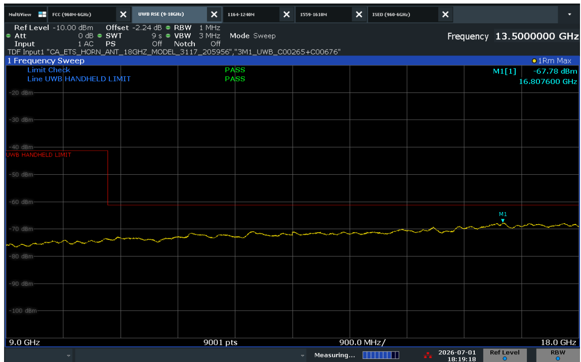
Plot 7-30. Radiated Spurious Emission 9-18GHz (Ch. 9, Config 9, Payload 125B Ant. Pol. V)
