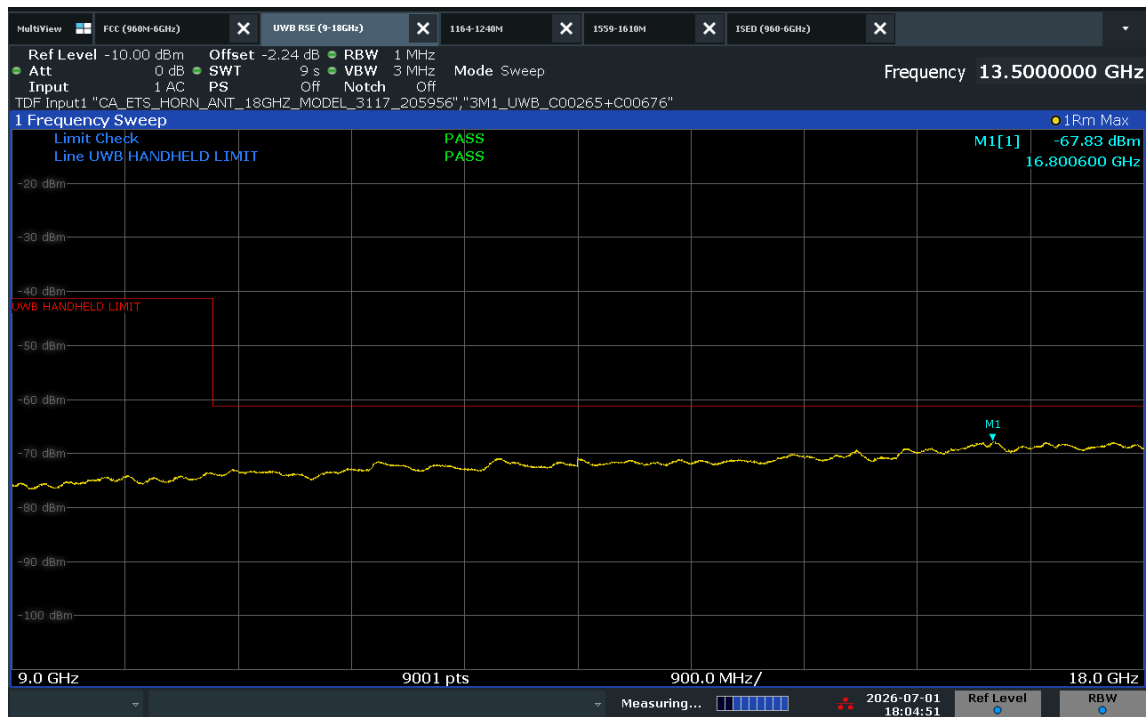
Plot 7-22. Radiated Spurious Emission 9-18GHz (Ch. 5, Config 9, Payload 125B Ant. Pol. V)
