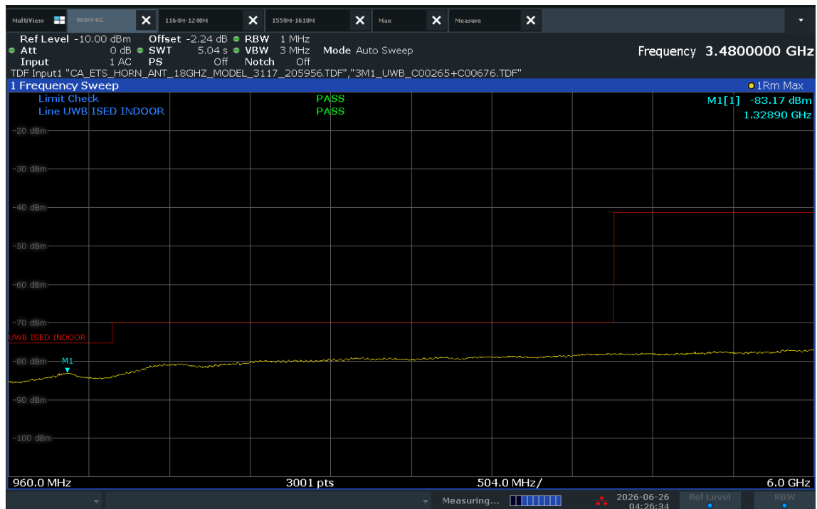
Plot 7-18. ISD Radiated Spurious Emission 960-6000MHz (Ch. 5, Config 9, Payload 125B Ant. Pol. V)
